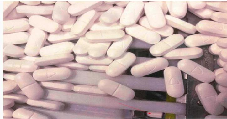
**Figure 11.** Tablet feed chute blockage (Cross-sectional view).
