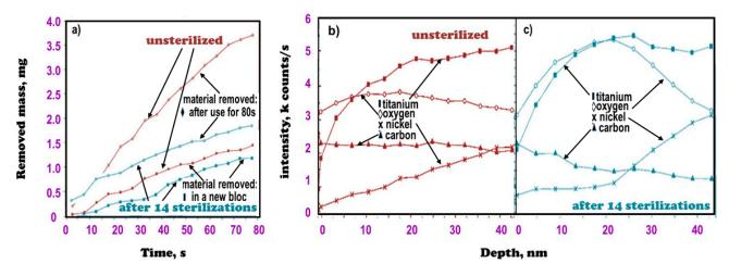
**Figure 6.** Properties of nitinol endodontic tools as delivered and after subsequent sterilization processes: (a) weight loss of the tool after drilling in a PMMA trial block with a simulated root canal used immediately after delivery or after repeated use for 80 s; (b,c) changes in the concentration of Ti, O, Ni, and C on the tool surface in the delivered condition (b) and after subsequent sterilization cycles (c).
