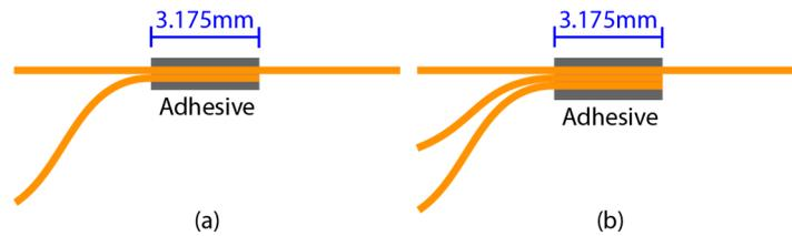
Figure 3. Sketch of the (a)  $2 \times 1$  and (b)  $3 \times 1$  acoustic coupler.
