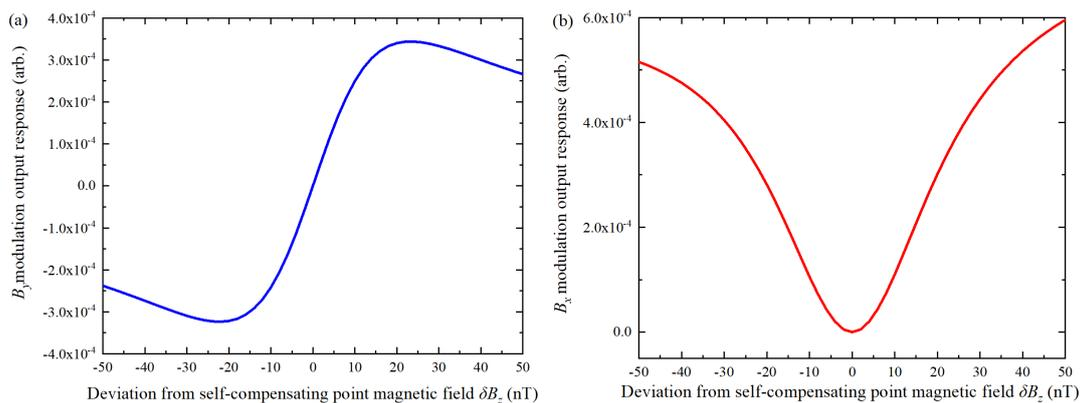
**Figure 1.**  $B_y$  and  $B_x$  step magnetic field modulation output response of SERF co-magnetometer. (a)  $B_y$  modulation output response at different residual magnetic fields. (b)  $B_x$  modulation output response at different residual magnetic fields.
