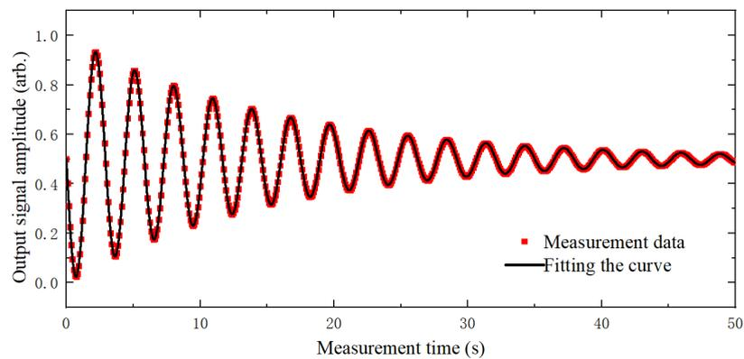
**Figure 5.** Experimental measurement of transverse relaxation rate of inert atoms in strongly coupled spin ensemble without magnetic field gradient.
