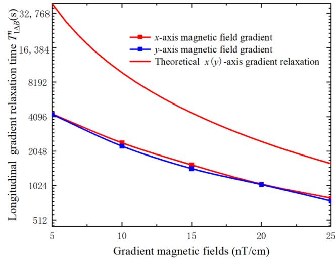
**Figure 7.** Measured relaxation times of the longitudinal magnetic gradient of inert atoms with an applied x- and y-axis magnetic field gradient, respectively, and curves calculated by the theoretical equations.
