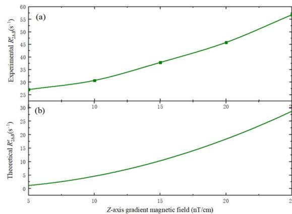
**Figure 4.** Experimental results of magnetic gradient relaxation of alkali metal atoms in coupled spin ensemble under applied *z*-axis magnetic gradient. (a) The experimental measurement results; (b) The simulation results based on the theoretical Equation (15).
