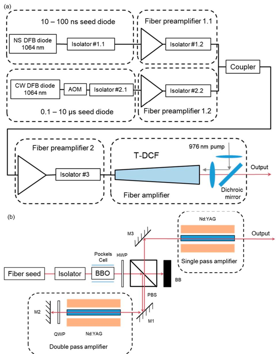
**Figure 1.** Experimental setup for hybrid laser system. (a) Fiber seed laser; (b) Nd:YAG rods amplifier. AOM: acousto-optic modulator; T-DCF: tapered double-clad fiber; HWP:  $\lambda/2$  wave plate; QWP:  $\lambda/4$  wave plate; PBS: polarization beam splitter; BB: beam blocker.
