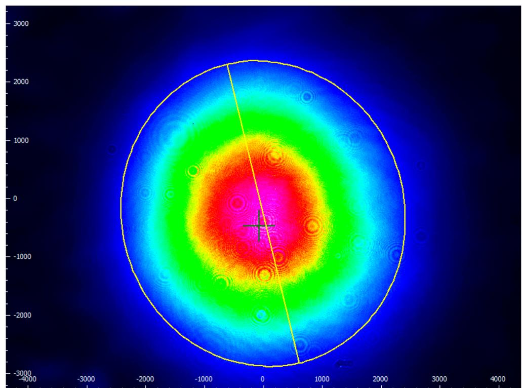
**Figure 3.** Resulting beam: near-field intensity profile.
