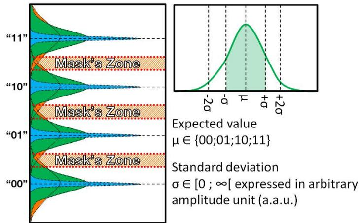
**Figure 2.** Gaussian noise representation on each PAM4 level for different standard deviations (blue: low standard deviation; green: medium; orange: high).
