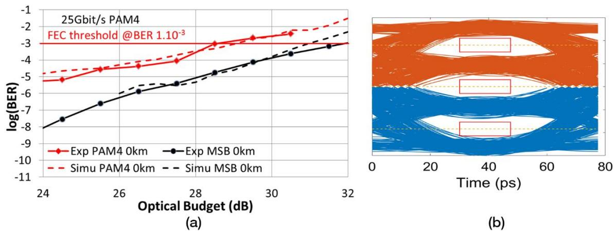
**Figure 4.** (a) Calibration of the simulation with experiment for PAM4 transmission in optical back to back at 25Gbit/s with a PRBS15; (b) Eye diagram with rectangular decision masks.
