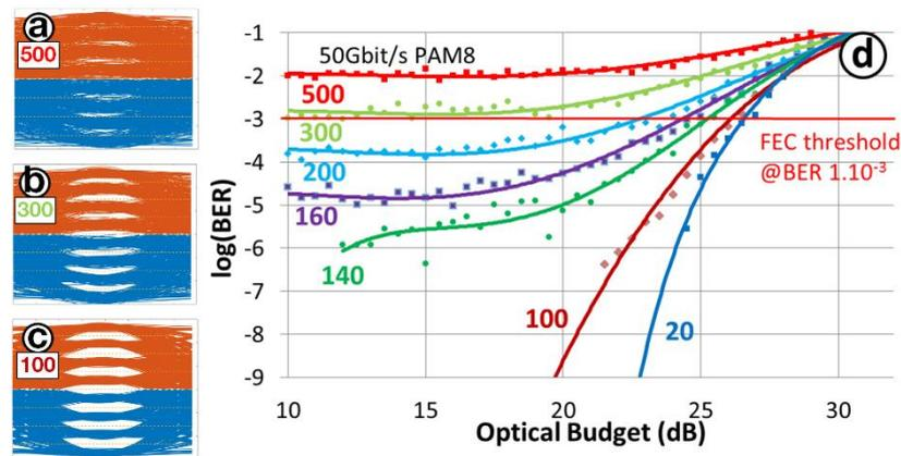
**Figure 6.** PAM8 eye diagrams for standard deviations of the decoder’s Gaussian noise of (a) 500 a.a.u., (b) 300 a.a.u., and (c) 100 a.a.u. (d) Simulated and polynomial approximations of BER versus Optical Budgets for different standard deviations of the simulated decoder’s noise.
