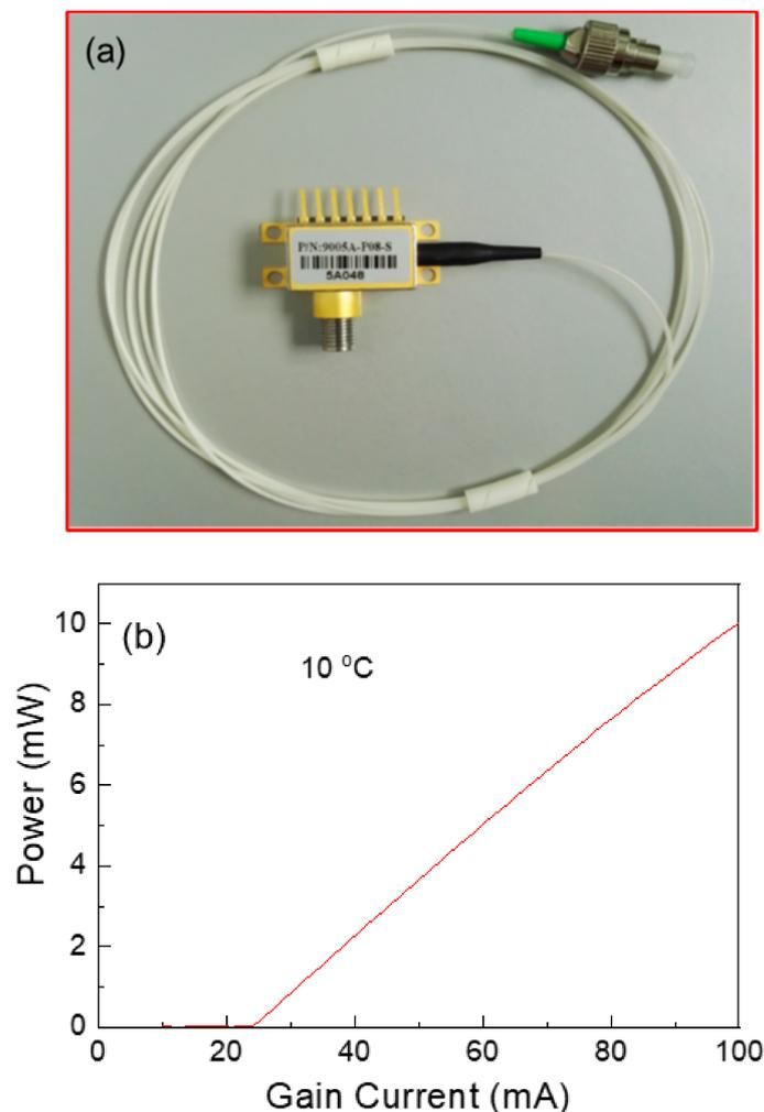
**Figure 1.** (a) Picture of a packaged distributed Bragg reflector (DBR) laser. (b) The light–current characteristic of the device at 10  $^{\circ}\text{C}$ .
