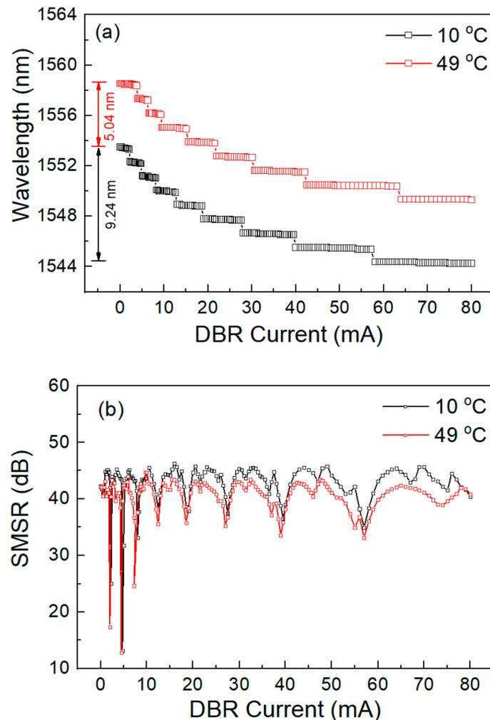
**Figure 2.** Laser emission wavelength (a) and sidemode suppression ratio (SMSR) (b) as functions of the injection current of the DBR section at a gain current of 80 mA at 10 and 49 °C, respectively.
