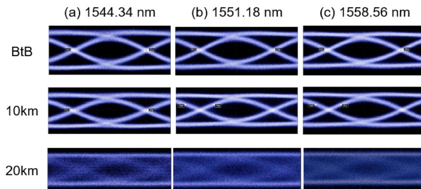
**Figure 6.** A 25 Gb/s eye diagram of a tunable DBR laser for BtB, 10 km, and 20 km transmission when the tuned wavelength is (a) 1544.34 nm, (b) 1551.18 nm, and (c) 1558.56 nm.
