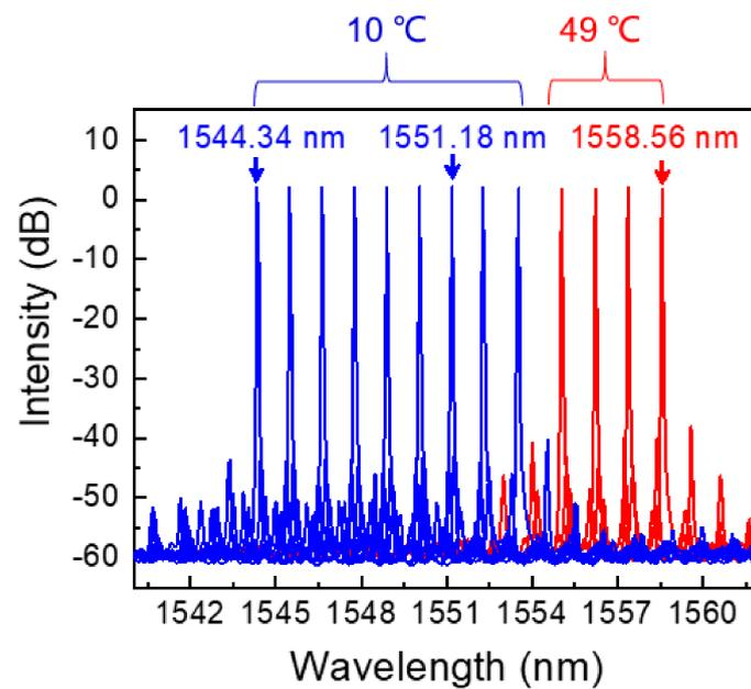
**Figure 3.** Typical optical spectra of the DBR laser at 10 and 49 °C.
