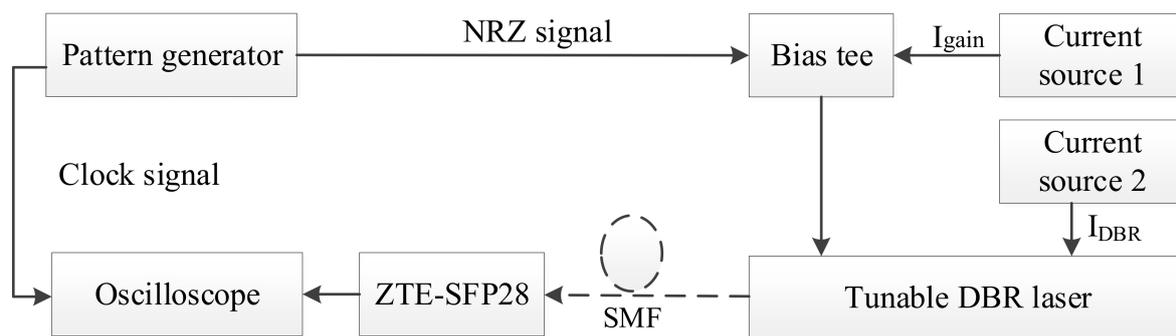
**Figure 5.** Experimental setup used to measure the 25 Gb/s transmission characteristics of the packaged DBR laser. NRZ: non-return-to-zero; SMF: single mode fiber; DBR: distributed Bragg reflector.
