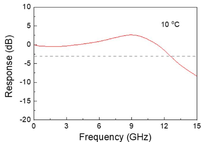
**Figure 4.** Small-signal modulation response at 10 °C when the gain section and DBR section were biased at 80 and 0 mA.
