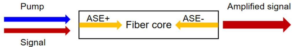
Figure 7. Propagation of the pump laser, signal laser and ASE in the Tm-doped fiber core.
