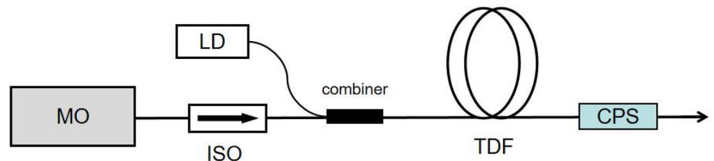
**Figure 2.** Layout of the all-fiber single-mode wavelength-tunable narrow-linewidth polarization-maintaining (PM) Tm-doped fiber power amplifier. MO: master-oscillator; LD: laser diode; TDF: Tm-doped fiber; ISO: isolator; CPS: cladding power stripper.
