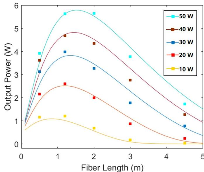
Figure 8. Relationship between amplified signal power and fiber length under different pump power. The solid line is calculated theoretically, and the square point is the experimental data.
