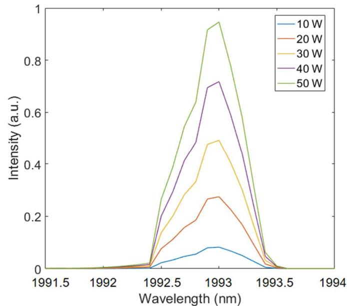
**Figure 9.** The change of signal laser spectrum under different pump power in 2 m optical fiber.
