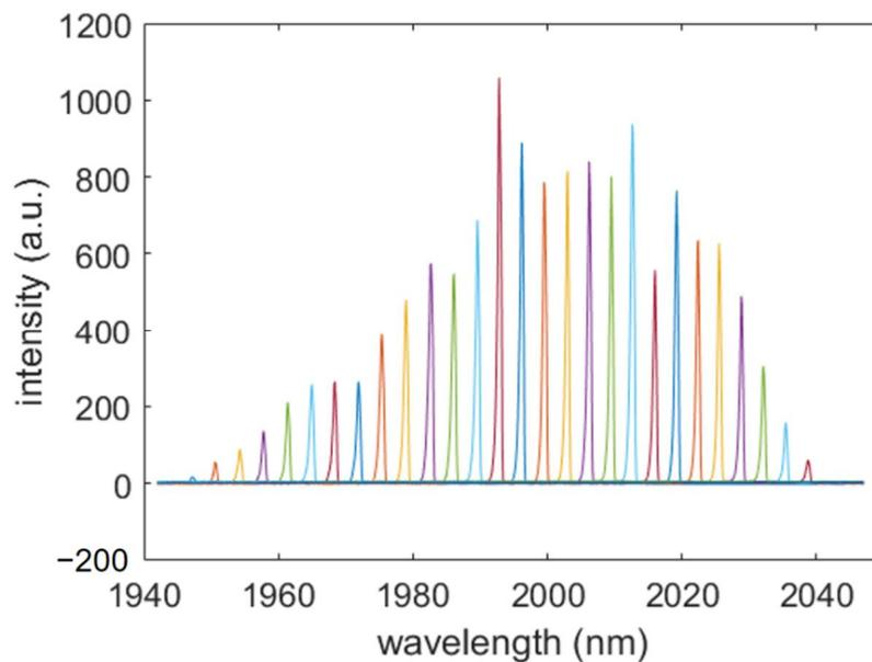
Figure 4. The spectrogram of the MOPA system.
