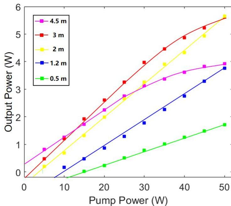
Figure 6. Variation of output power with pump power under different fiber lengths in the PA system.
