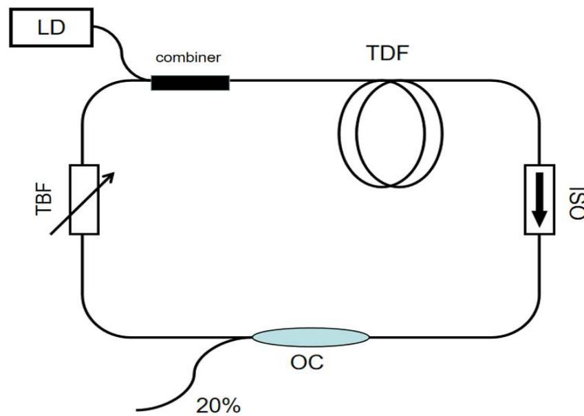
**Figure 1.** Layout of the all-fiber single-mode wavelength-tunable narrow-linewidth polarization-maintaining (PM) Tm-doped fiber master oscillator. LD: laser diode; TDF: Tm-doped fiber. ISO: isolator; OC: optical coupler; TBF: tunable band-pass filter.
