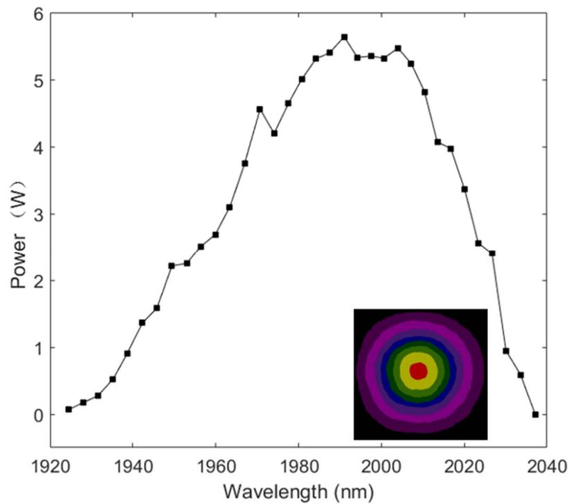
Figure 3. The output power of the MOPA system.
