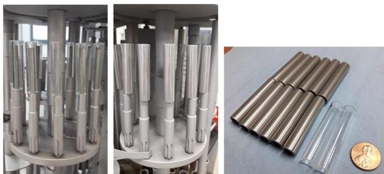
**Figure 13.** Raschig rings prepared for the PVD process (left), and substrates after arc-PVD  $\text{TiO}_x$  deposition (middle and right).
