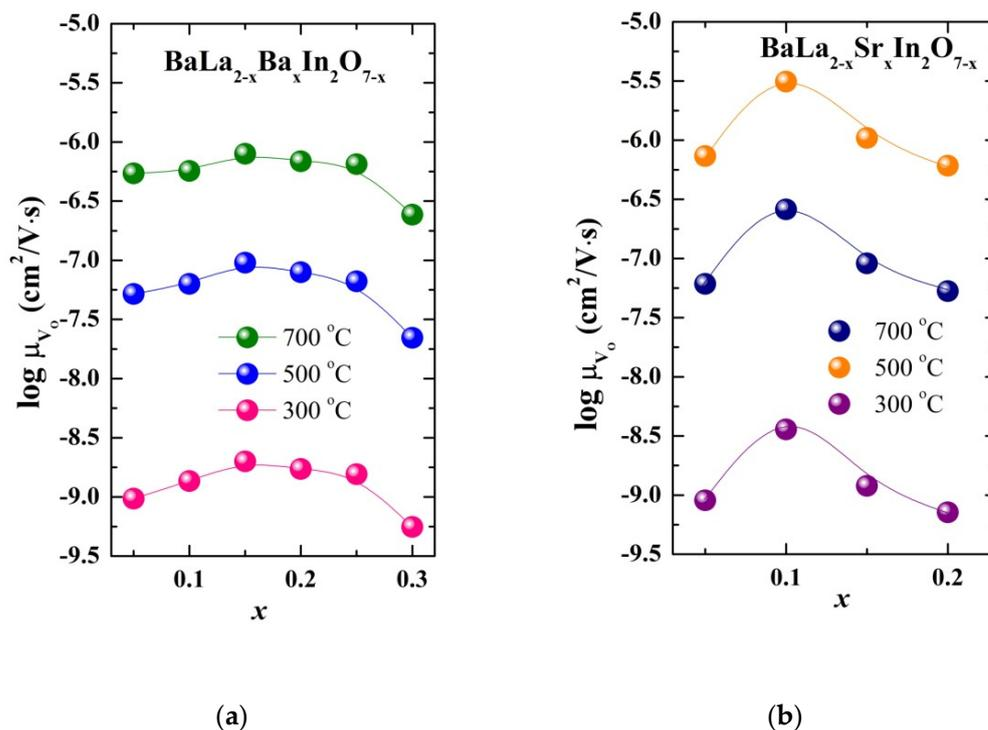
**Figure 8.** The concentration dependencies of oxygen ions mobility at 700, 500, and 300 °C for the solid solutions  $\text{BaLa}_{2-x}\text{Ba}_x\text{In}_2\text{O}_{7-0.5x}$  (a) and  $\text{BaLa}_{2-x}\text{Sr}_x\text{In}_2\text{O}_{7-0.5x}$  (b).
