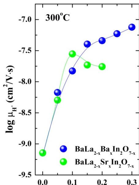
**Figure 10.** The concentration dependencies of oxygen ions mobility at 300 °C for the solid solutions  $\text{BaLa}_{2-x}\text{Ba}_x\text{In}_2\text{O}_{7-0.5x}$  and  $\text{BaLa}_{2-x}\text{Sr}_x\text{In}_2\text{O}_{7-0.5x}$ .
