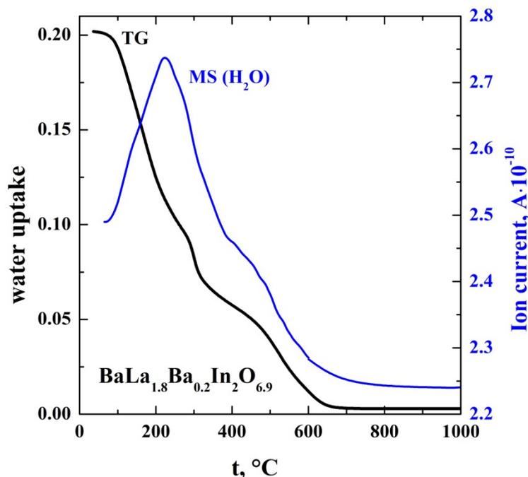
Figure 3. The TG and MS(H<sub>2</sub>O) curves of BaLa<sub>1.8</sub>Ba<sub>0.2</sub>In<sub>2</sub>O<sub>6.9</sub>·0.2H<sub>2</sub>O composition.
