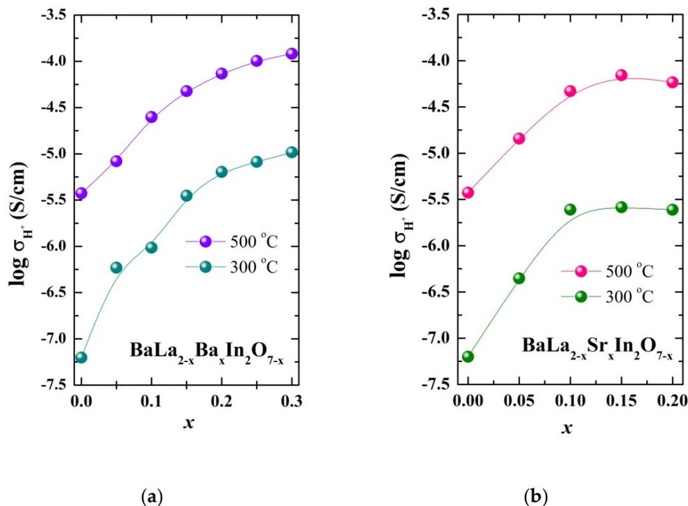
**Figure 9.** The concentration dependencies of proton conductivity at 500 and 300 °C for the solid solutions  $BaLa_{2-x}Ba_xIn_2O_{7-0.5x}$  (a) and  $BaLa_{2-x}Sr_xIn_2O_{7-0.5x}$  (b).
