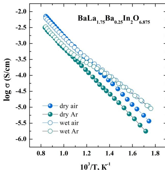
**Figure 4.** The temperature dependencies of conductivity for the composition  $\text{BaLa}_{1.75}\text{Ba}_{0.25}\text{In}_2\text{O}_{6.875}$  under dry (filled symbols) and wet (open symbols) conditions.
