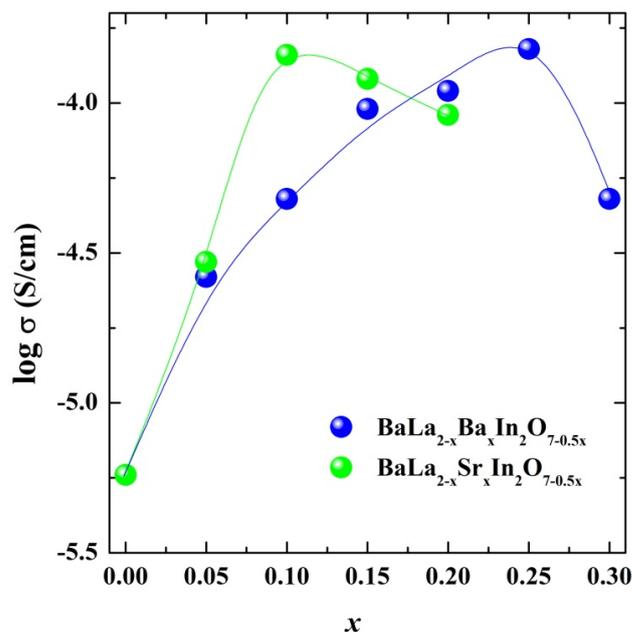
**Figure 5.** The concentration dependencies of electrical conductivity at 500 °C under dry air for the solid solutions  $BaLa_{2-x}M_xIn_2O_{7-0.5x}$  ( $M = Sr, Ba$ ).
