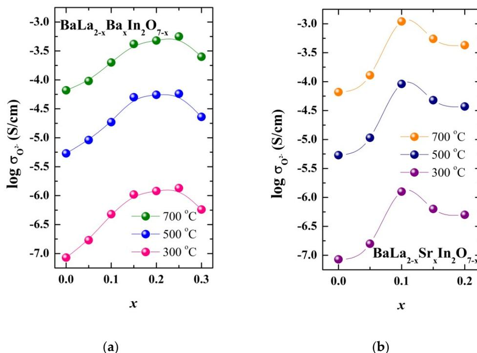
**Figure 7.** The concentration dependencies of oxygen ion conductivity at 300, 500, and 700 °C for the solid solutions  $\text{BaLa}_{2-x}\text{Ba}_x\text{In}_2\text{O}_{7-0.5x}$  (a) and  $\text{BaLa}_{2-x}\text{Sr}_x\text{In}_2\text{O}_{7-0.5x}$  (b).
