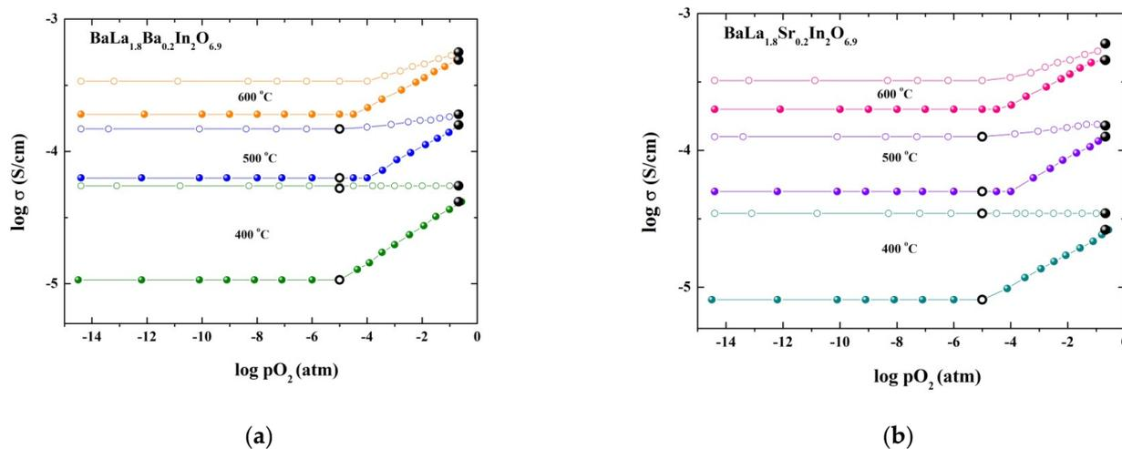
**Figure 6.** The dependencies of the conductivity values vs. oxygen partial pressure for the compositions  $BaLa_{1.8}Ba_{0.2}In_2O_{6.9}$  (a) and  $BaLa_{1.8}Sr_{0.2}In_2O_{6.9}$  (b) under dry (filled symbols) and wet (open symbols) conditions and conductivity values from  $\sigma$ – $10^3/T$  dependencies under wet air (filled black symbols) and wet Ar (open black symbols) conditions.
