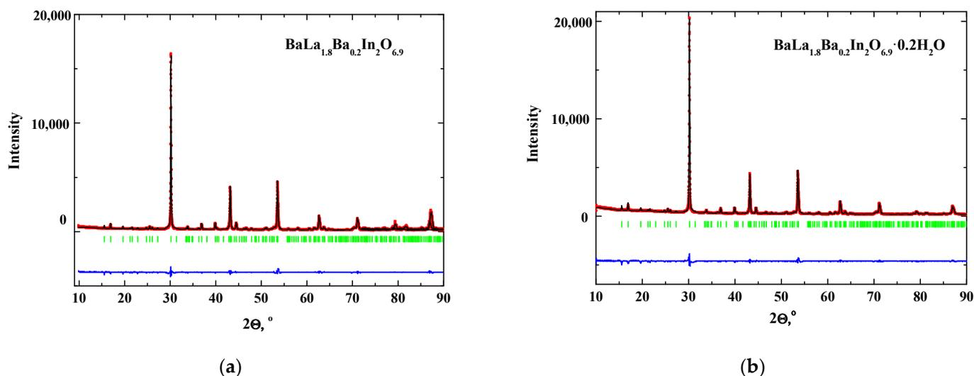
**Figure 2.** The XRD data for the anhydrous  $\text{BaLa}_{1.8}\text{Ba}_{0.2}\text{In}_2\text{O}_{6.9}$  (a) and hydrated  $\text{BaLa}_{1.8}\text{Ba}_{0.2}\text{In}_2\text{O}_{6.9}\cdot 0.2\text{H}_2\text{O}$  (b) compositions.
