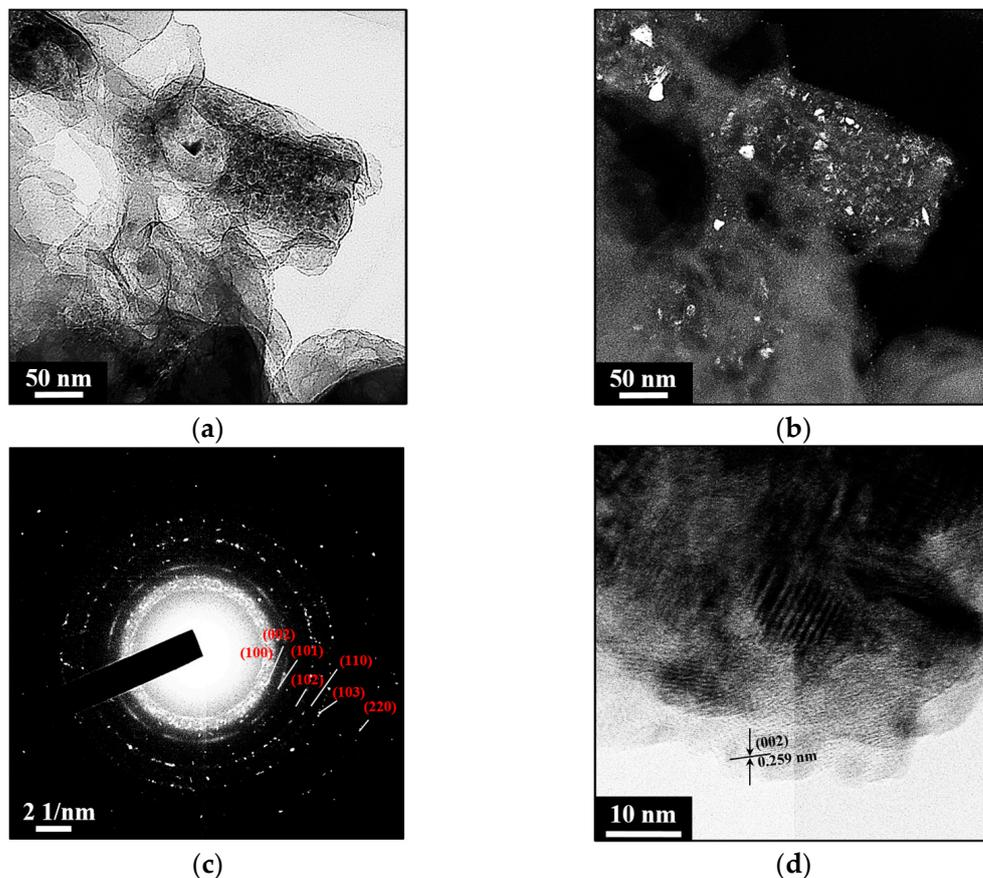
**Figure 4.** (a) The bright-field and (b) dark-field transmission electron microscopy (TEM) image of  $g\text{-C}_3\text{N}_4/7.5\% \text{ ZnO}$  NPs, (c) selected area electron diffraction (SAED) pattern, and (d) high resolution-TEM (HR-TEM) image.
