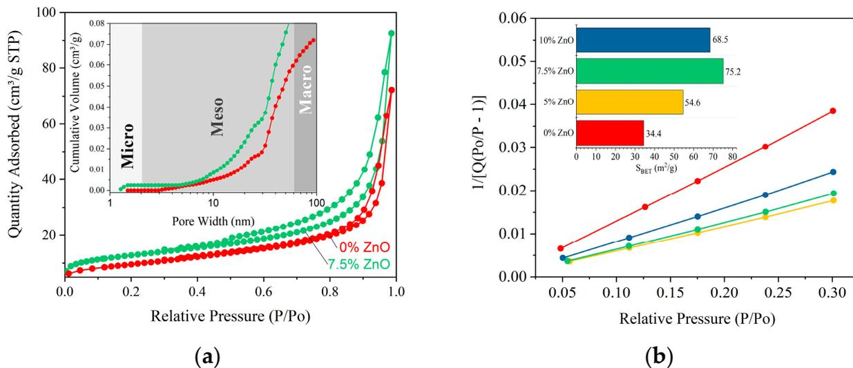
**Figure 5.** (a)  $\text{N}_2$  adsorption-desorption isotherms of initial  $g\text{-C}_3\text{N}_4$  and  $g\text{-C}_3\text{N}_4/7.5\% \text{ ZnO}$  samples; (b) BET surface area plot of initial  $g\text{-C}_3\text{N}_4$  and  $g\text{-C}_3\text{N}_4/\text{ZnO}$  nanocomposites.
