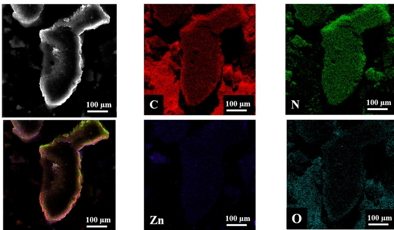
**Figure 3.** EDX mapping of  $g\text{-C}_3\text{N}_4/7.5\%$  ZnO nanocomposite.
