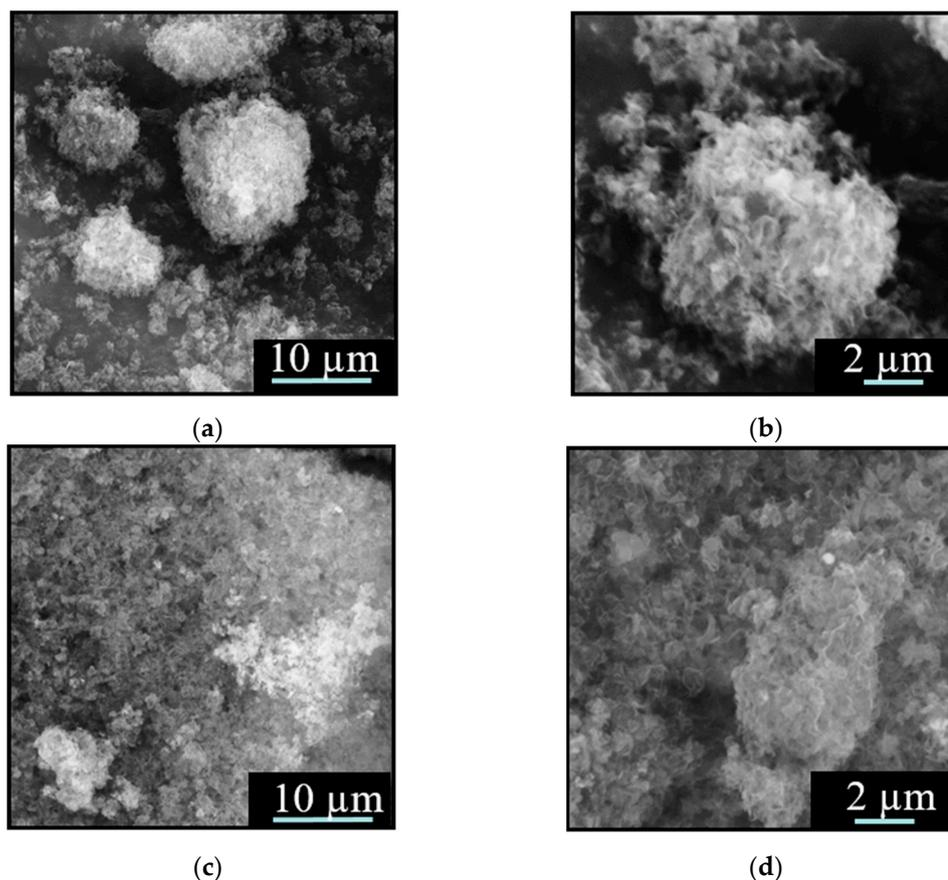
**Figure 2.** SEM images of (a,b) pure  $g\text{-C}_3\text{N}_4$  and (c,d)  $g\text{-C}_3\text{N}_4/7.5\%$  ZnO.
