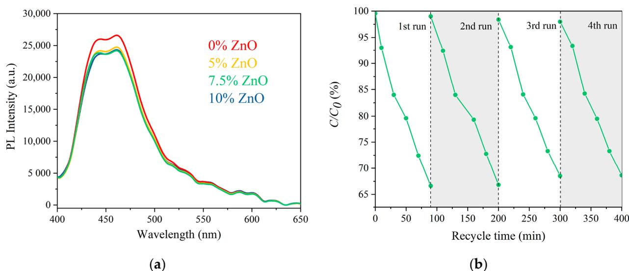
**Figure 8.** (a) PL spectra of initial g-C<sub>3</sub>N<sub>4</sub> and g-C<sub>3</sub>N<sub>4</sub>/ZnO (5% ZnO, 7.5% ZnO and 10% ZnO) nanocomposites; (b) Recycling photocatalytic test of g-C<sub>3</sub>N<sub>4</sub>/7.5% ZnO.
