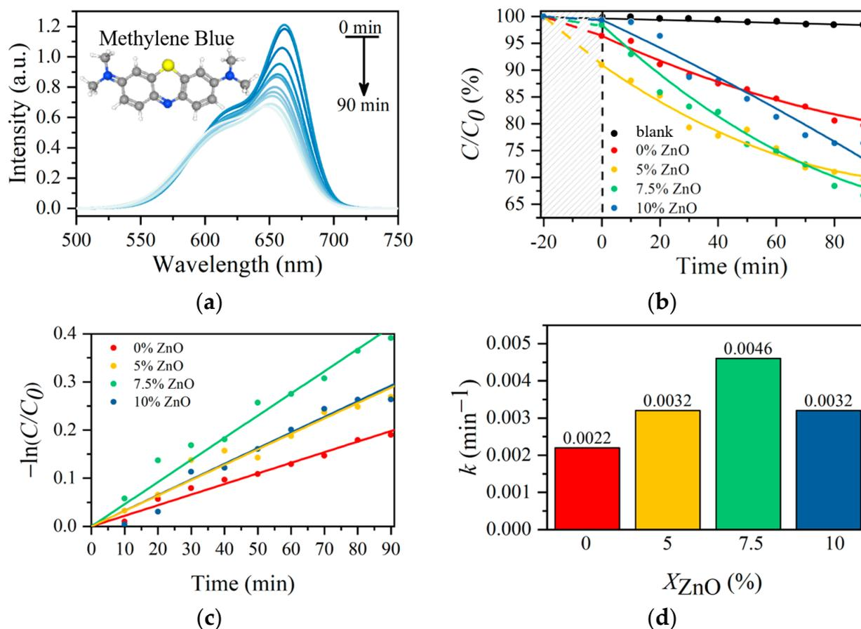
**Figure 7.** (a) Photocatalytic degradation of MB over  $g\text{-C}_3\text{N}_4/7.5\%$  ZnO catalyst under visible light; (b) Kinetic curves, (c) Logarithmic kinetic curves of the pseudo-first-order process; (d) Photodecomposition rate constant versus ZnO content.
