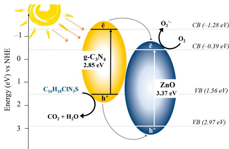
**Figure 9.** Schematic mechanism of photocatalytic degradation of MB of g-C<sub>3</sub>N<sub>4</sub>/ZnO under visible light.
