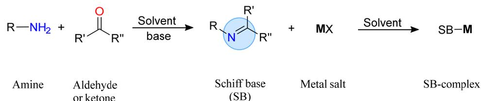
**Scheme 1.** General synthesis of Schiff Bases Complexes.
