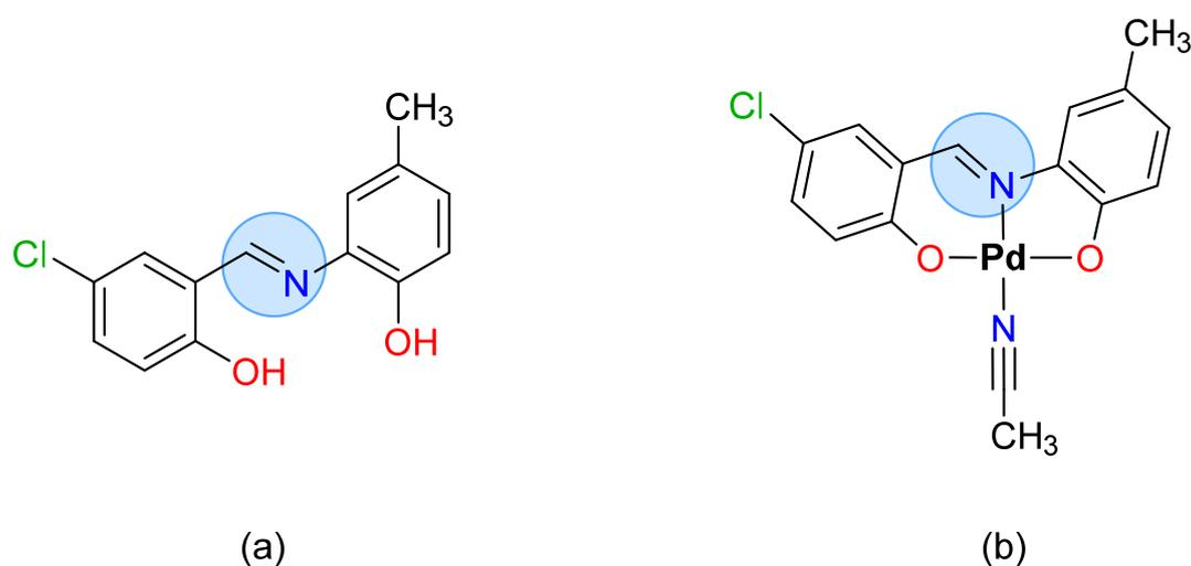
**Figure 2.** Structure of (a) tridentate Schiff base and (b) its palladium pincer complex with antimicrobial activity.
