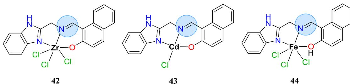
**Figure 19.** Zr(IV), Cd(II), and Fe(III) complexes with a Schiff base synthesized from 2-aminomethylbenzimidazole and 2-hydroxynaphthaldehyde.
