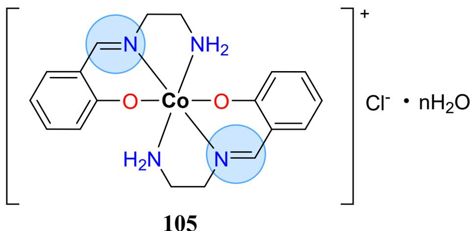
**Figure 54.** Co(III) complex with a tridentate SB ligand derived from salicylaldehyde and ethylenediamine tested as antimicrobial agent.
