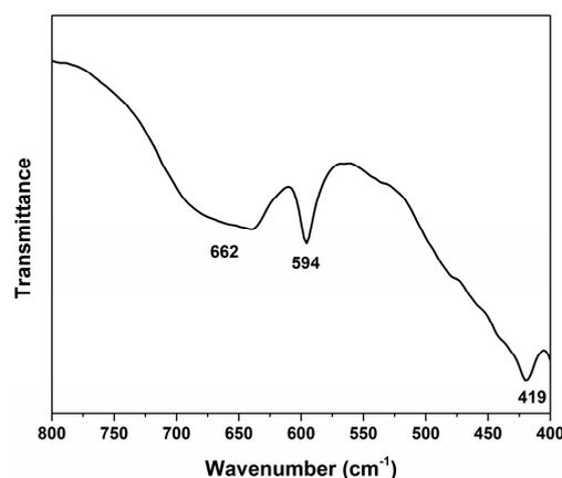
**Figure 3.** FT-IR spectrum of YMnO<sub>3</sub> sample synthesized at 1100 °C.
