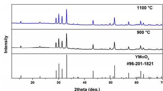
**Figure 2.** XRD patterns of  $\text{YMnO}_3$ , prepared at 900 °C and 1100 °C with the molar ratio between nitrates and chlorides as 1:2 with reaction time of 10 h.
