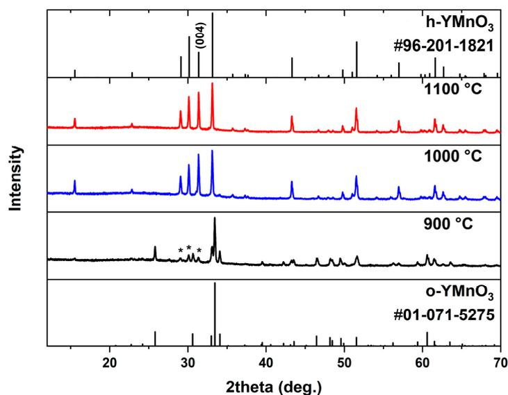
**Figure 5.** XRD patterns of  $\text{YMnO}_3$  prepared at different temperatures with the molar ratio between precursors and chlorides 1:10. \* represents the peaks belonging to the h- $\text{YMnO}_3$ .
