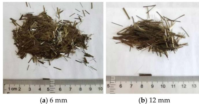
Figure 11. Basalt fiber.
