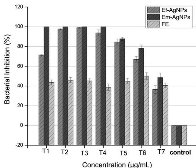
**Figure 6.** Inhibition of *Erwinia carotovora* subsp. *carotovora* by extract-free silver nanoparticles (Ef-AgNPs), extract-mixed silver nanoparticles (Em-AgNPs), and fruit extract (FE) of *Hedera nepalensis*. Concentrations (µg/mL) (T1:1000, T2: 500, T3: 250, T4: 125, T5: 62, T6: 31.25, T7: 15.62). The error bars indicate standard error of mean, and values are mean  $\pm$  standard error of three replicates.
