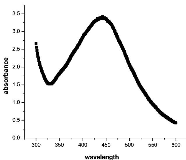
**Figure 1.** UV-vis absorbance spectrum of 6 mM  $\text{AgNO}_3$  and 5 mg/mL of *Hedera nepalensis* fruit extract mixed in 1:1 ( $v/v$ ) ratio.
