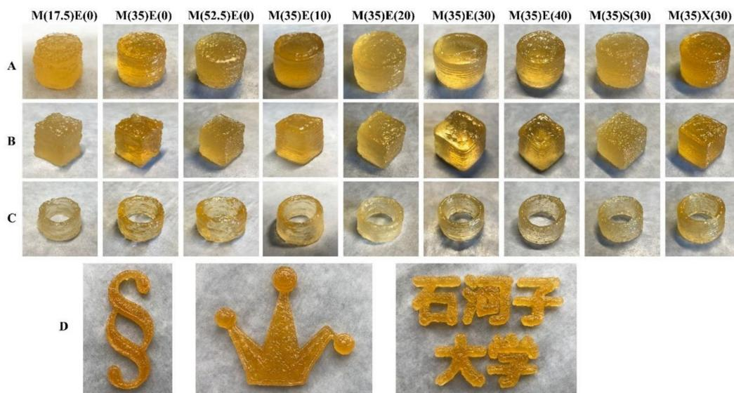
**Figure 1.** Printing performance with different formulation inks. (A) Solid cylinders with diameter of 15 mm and height of 15 mm. (B) Cubes with side length of 10 mm. (C) Hollow cylinders with wall thickness of 2 mm and height of 15 mm. (D) Gummies of different shapes printed with gummy ink.
