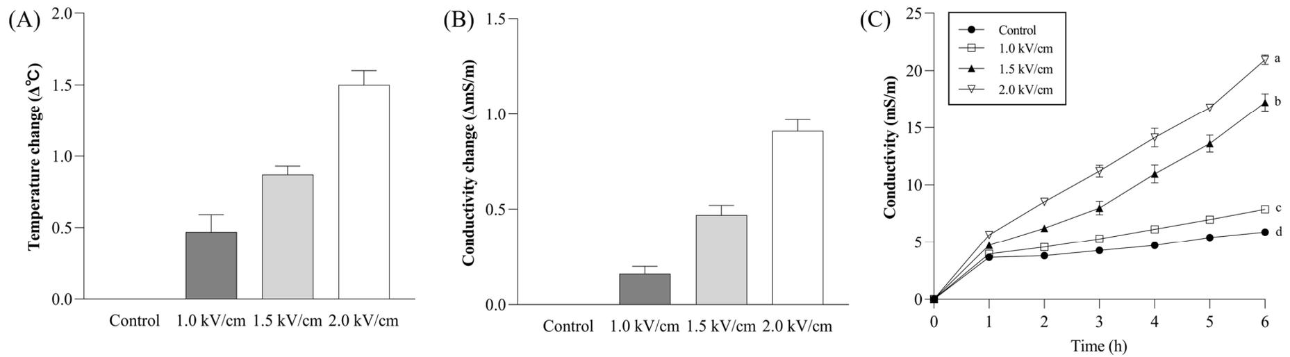
**Figure 1.** Effect of PEF treatment on the (A) temperature change, (B) conductivity change, and (C) ion release from tea leaves. The meanings of the symbols in the figure: ●—Control, □—1.0 kV/cm, ▲—1.5 kV/cm, ▽—2.0 kV/cm. All values are expressed by mean  $\pm$  SD ( $n = 3$ ). Values with different letters (a–d) are significantly different ( $p < 0.05$ ), as determined by Duncan's test.
