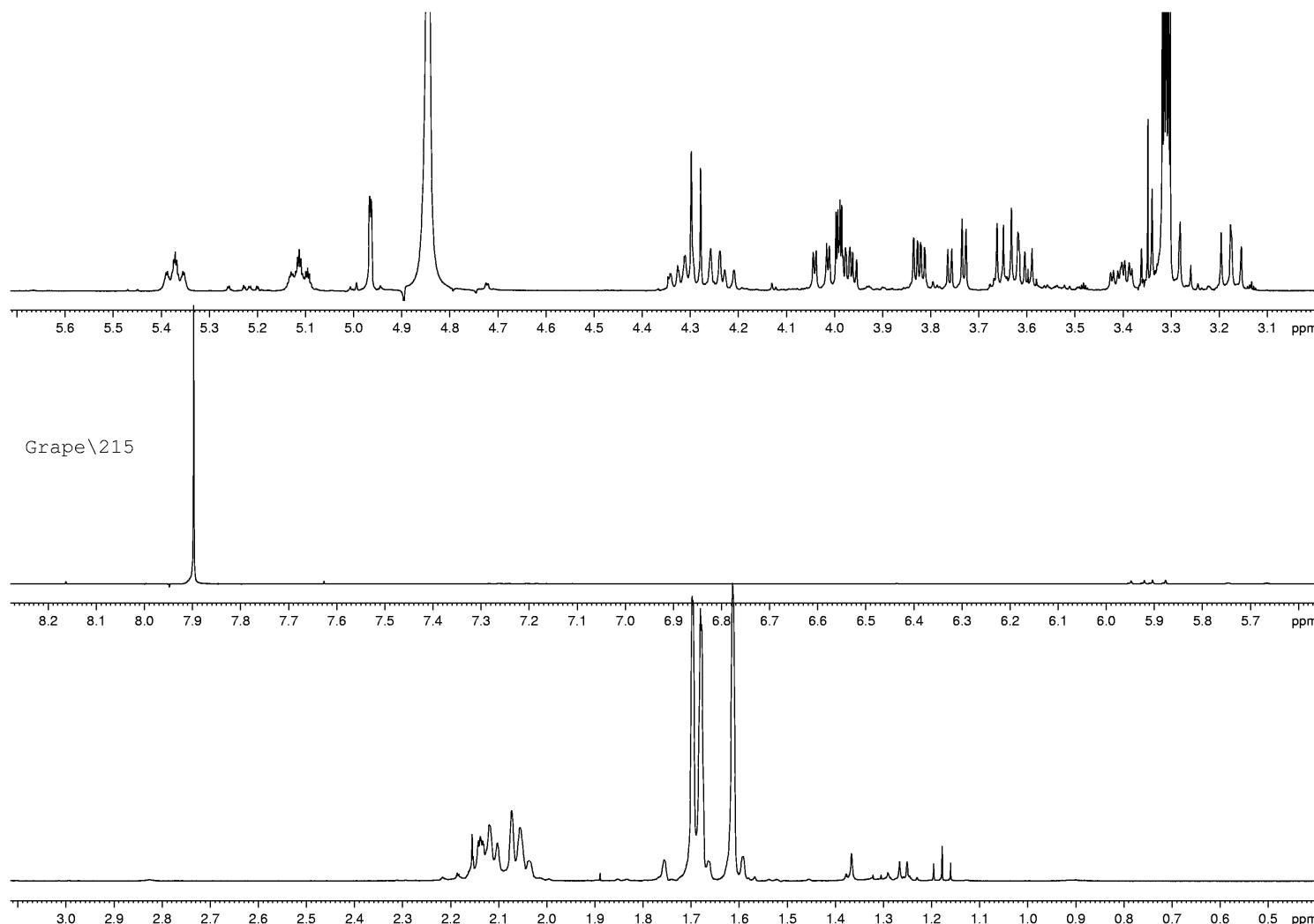
**Fig. S7.** The  $^1\text{H}$ -NMR spectrum of **9**
