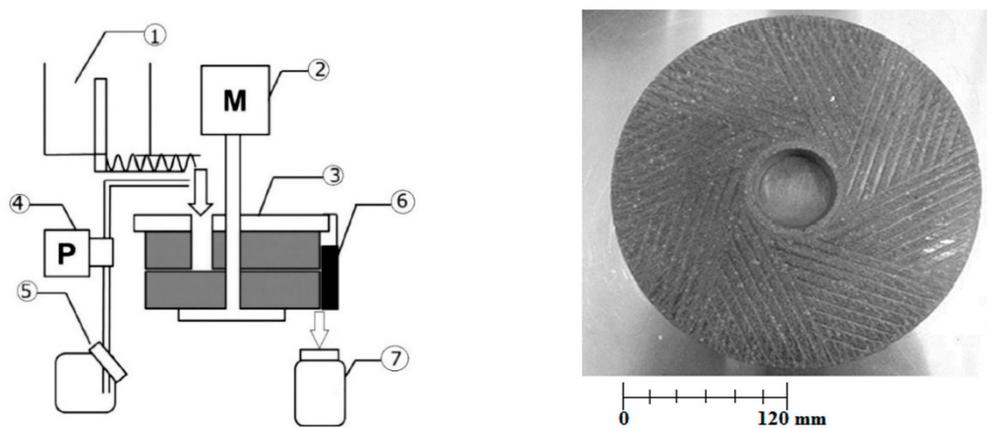
**Figure 1.** Schematic diagram of the micro wet milling system. (1) Rotary rice feeding equipment, (2) Motor, (3) Milling stone, (4) Tubing pump, (5) Water tank, (6) Rubber Spatula, (7) Receiver. Picture of the lower stone of mill [14].
