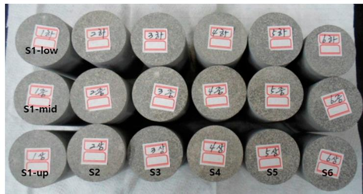
**Figure 3.** Image of polished representative samples collected from waste-form drums.
