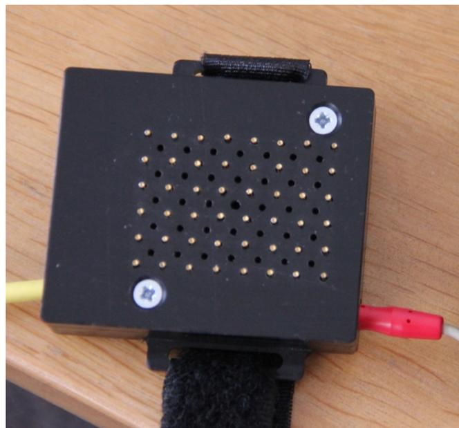
**Figure 2.** Application of the GEDIS system with a contact pressure of 15 N. The grounding electrode can be seen on the right.
