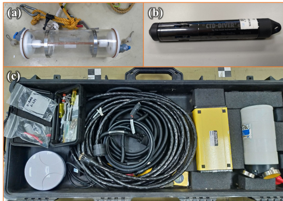
Figure 2. Instrumentation photographs (a) water collector, (b) conductivity–temperature–depth (CTD) sensor, and (c) acoustic Doppler current profiler (ADCP).
