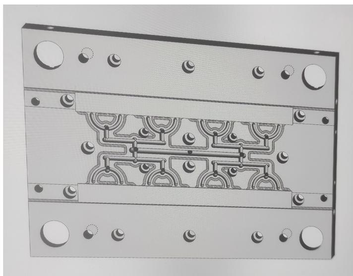
**Figure 1.** Cold runner injection mold type.
