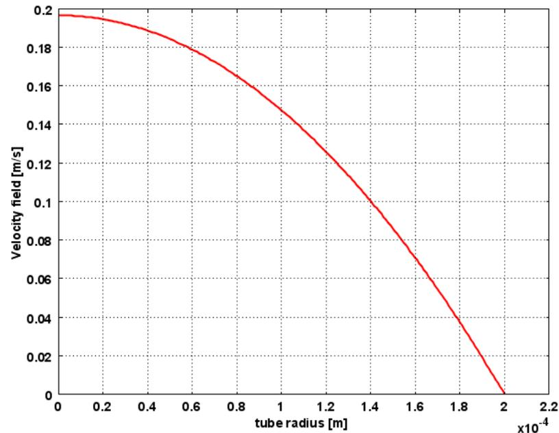
Figure 6. Flow velocity profile inside the tube.
