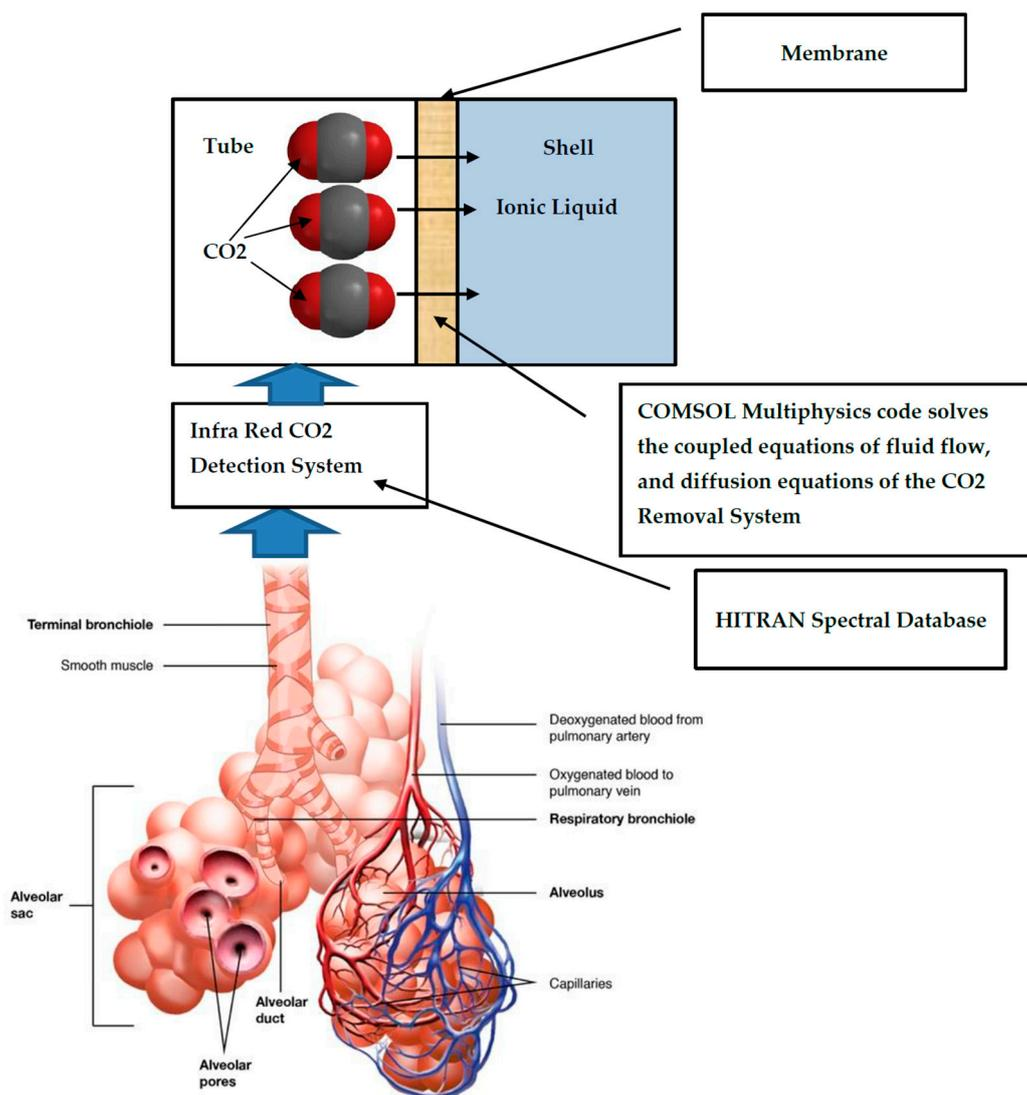
**Figure 2.** Schematics of the carbon dioxide removal system.
