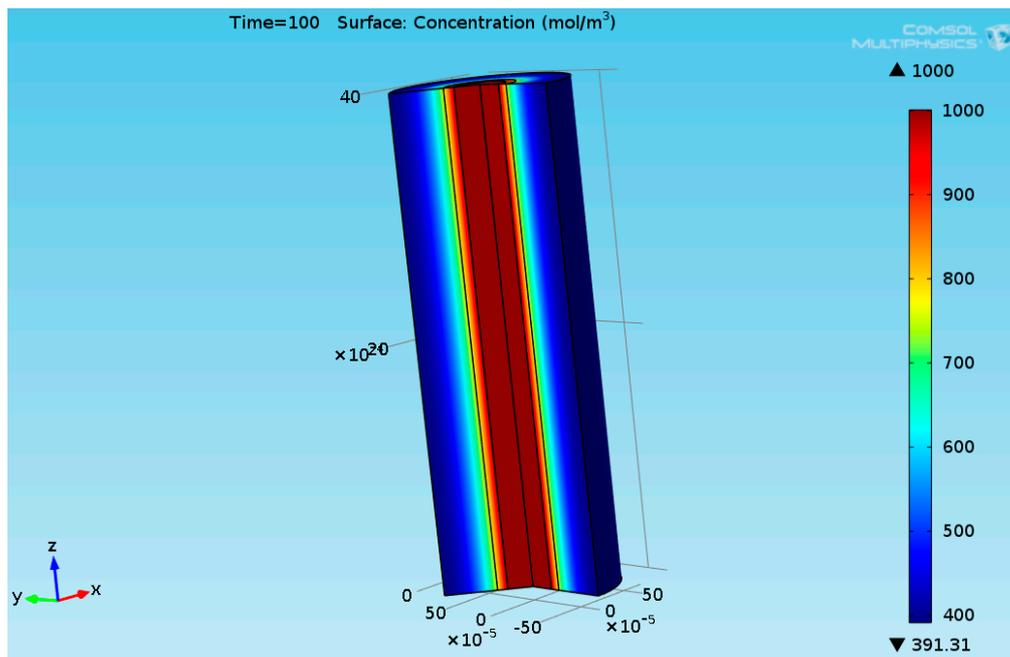
Figure 8. Three-dimensional plot of the carbon dioxide concentration profile.
