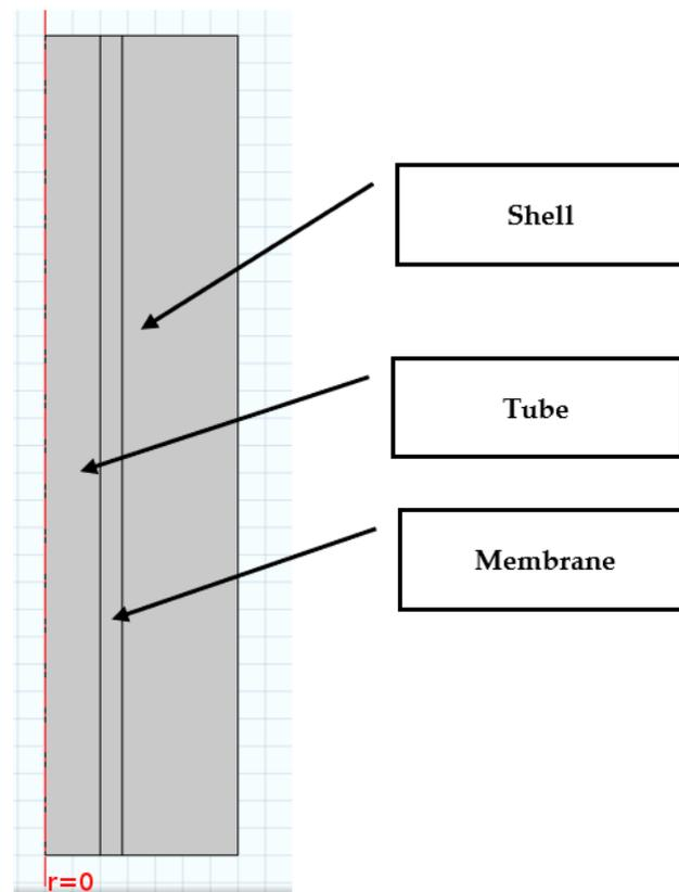
**Figure 3.** 2D plot of the carbon removal device.
