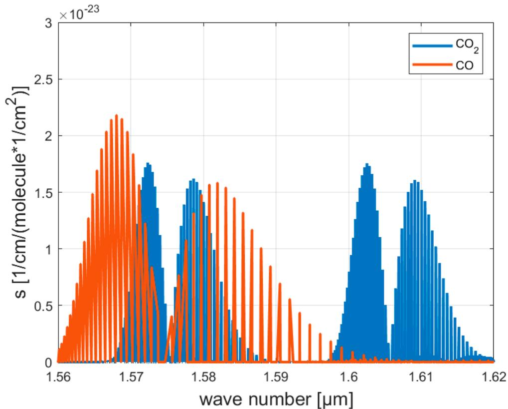
**Figure 4.** Calculated absorption spectra of gas columns with pure CO<sub>2</sub> and pure CO.
