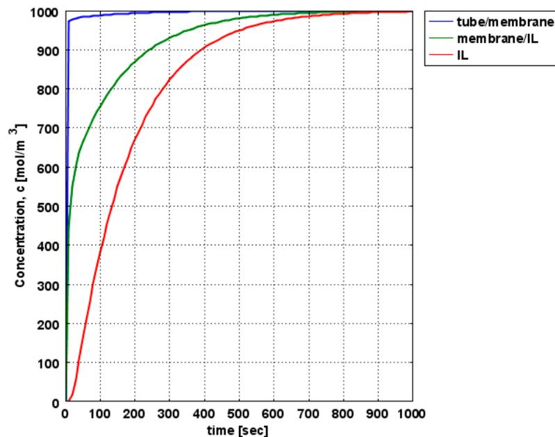
Figure 9. CO<sub>2</sub> concentrations at the different points of the carbon removal system (1640 elements).
