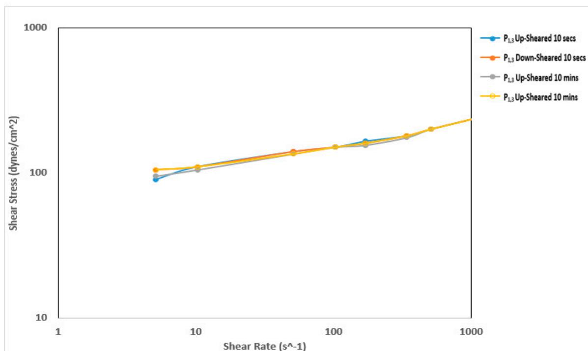
**Figure 8.** Thixotropy behavior of the mud prepared with Pindinga clay after thermochemical treatment.
