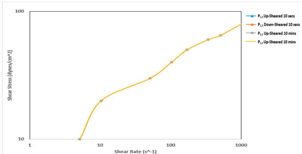
**Figure 7.** Thixotropy behavior of the mud prepared with Pindinga clay before thermochemical treatment.
