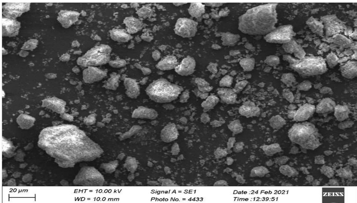
Figure 2. SEM Images of the raw clay material from Ubakala.
