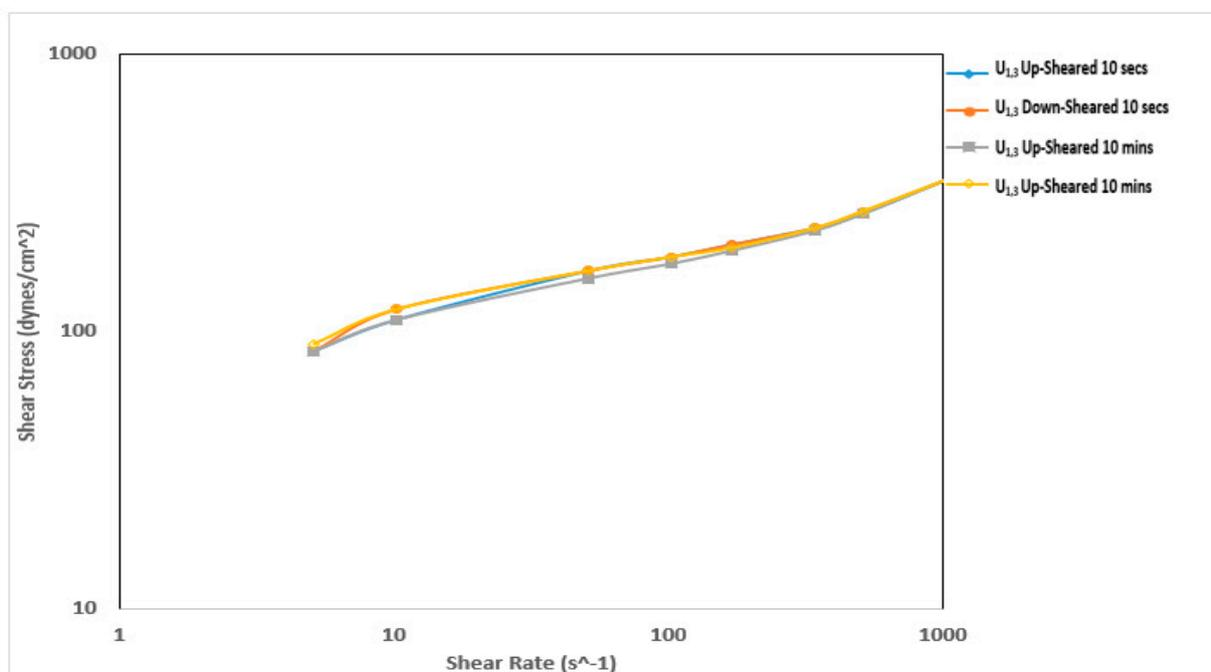
Figure 10. Thixotropy behavior of the mud prepared with Ubakala clay after thermochemical treatment.
