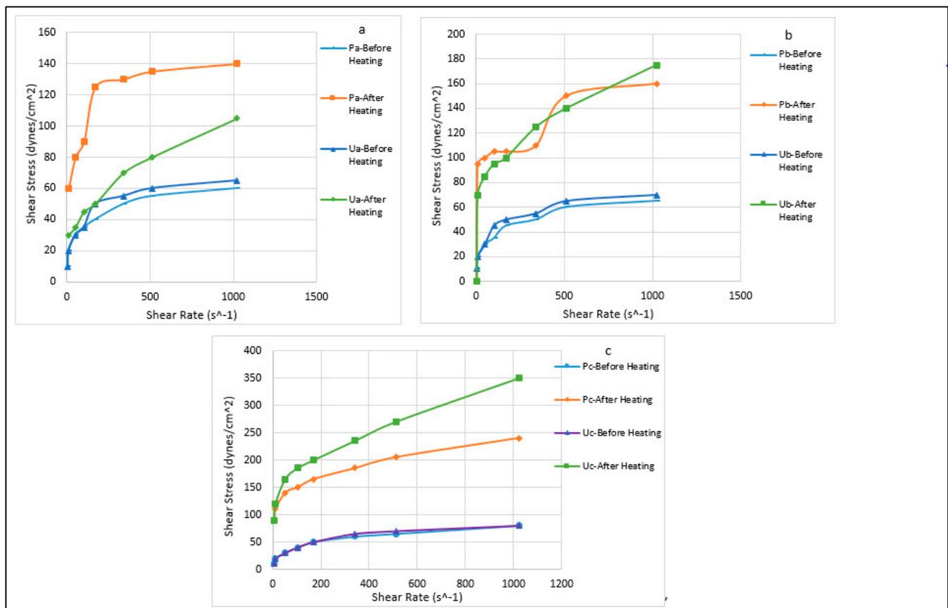
**Figure 6.** Effect of the thermochemical treatment on the shear stress to shear rate relationship of the mud samples: (a). Samples P<sub>1,3</sub> and U<sub>1,3</sub>. (b). Samples P<sub>2,3</sub> and U<sub>2,3</sub>. (c). Samples P<sub>3,3</sub> and U<sub>3,3</sub>.
