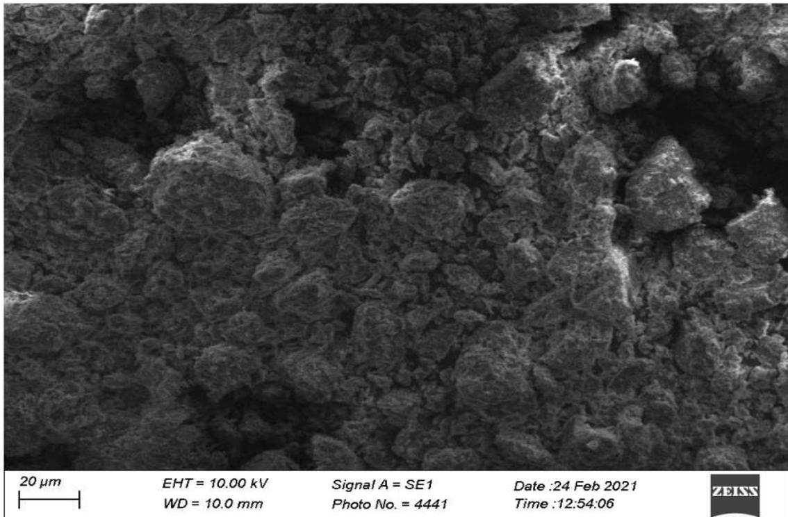
Figure 1. SEM Images of the raw clay material from Pindinga.
