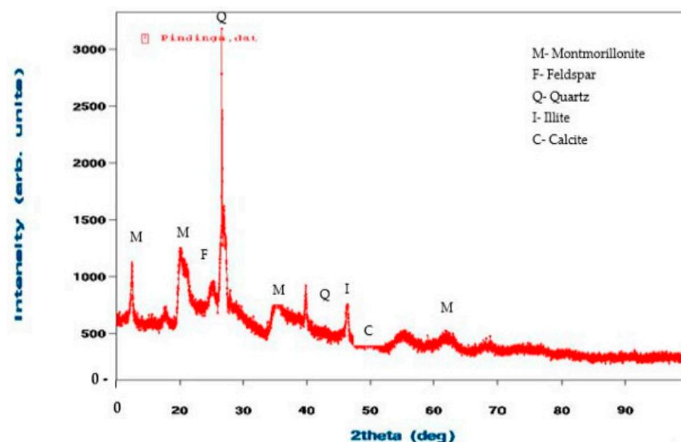
**Figure 3.** XRD Images of the raw clay material from Pindinga.
