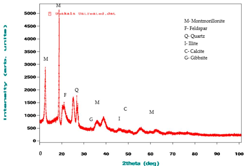
Figure 4. XRD Images of the raw clay material from Ubakala.
