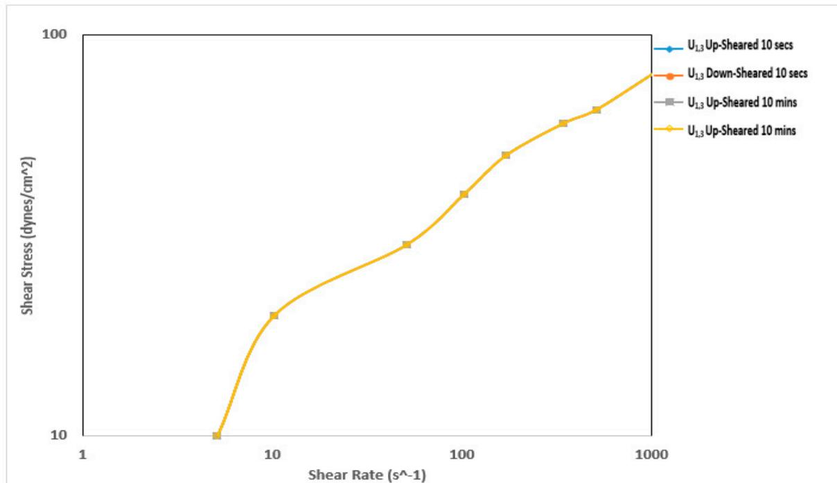
Figure 9. Thixotropy behavior of the mud prepared with Ubakala clay before thermochemical treatment.
