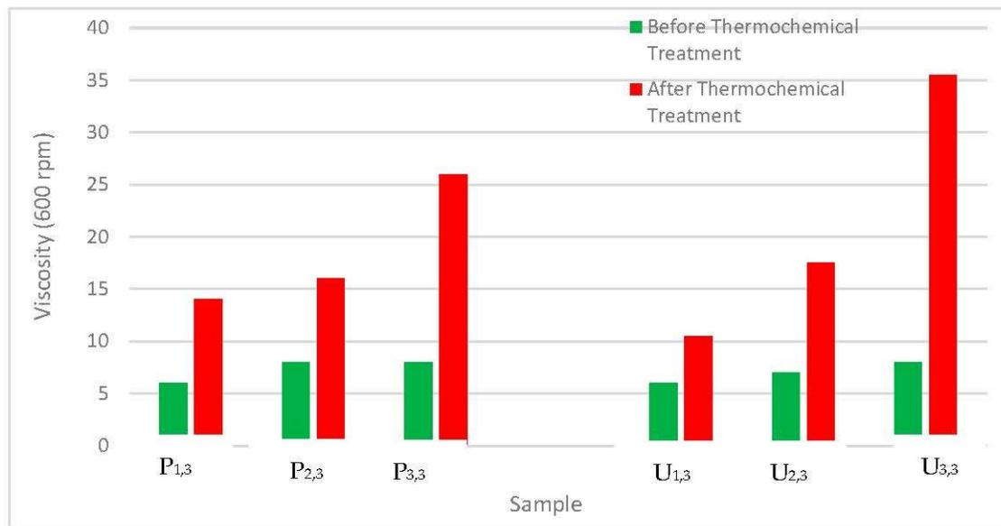
**Figure 5.** Effect of the thermochemical treatment of the local raw clay materials on the mud viscosity at 600 rpm.
