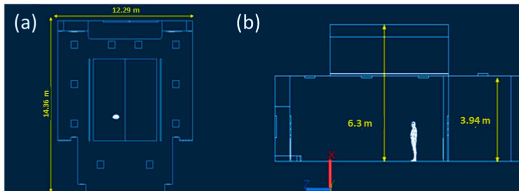
**Figure 1.** Characteristic measurements of Classroom C at the University of Naples Federico II. The top view shows maximum width and length (a), the side view shows average and maximum wall height (b) and was drawn with Autodesk Autocad 2021 software.
