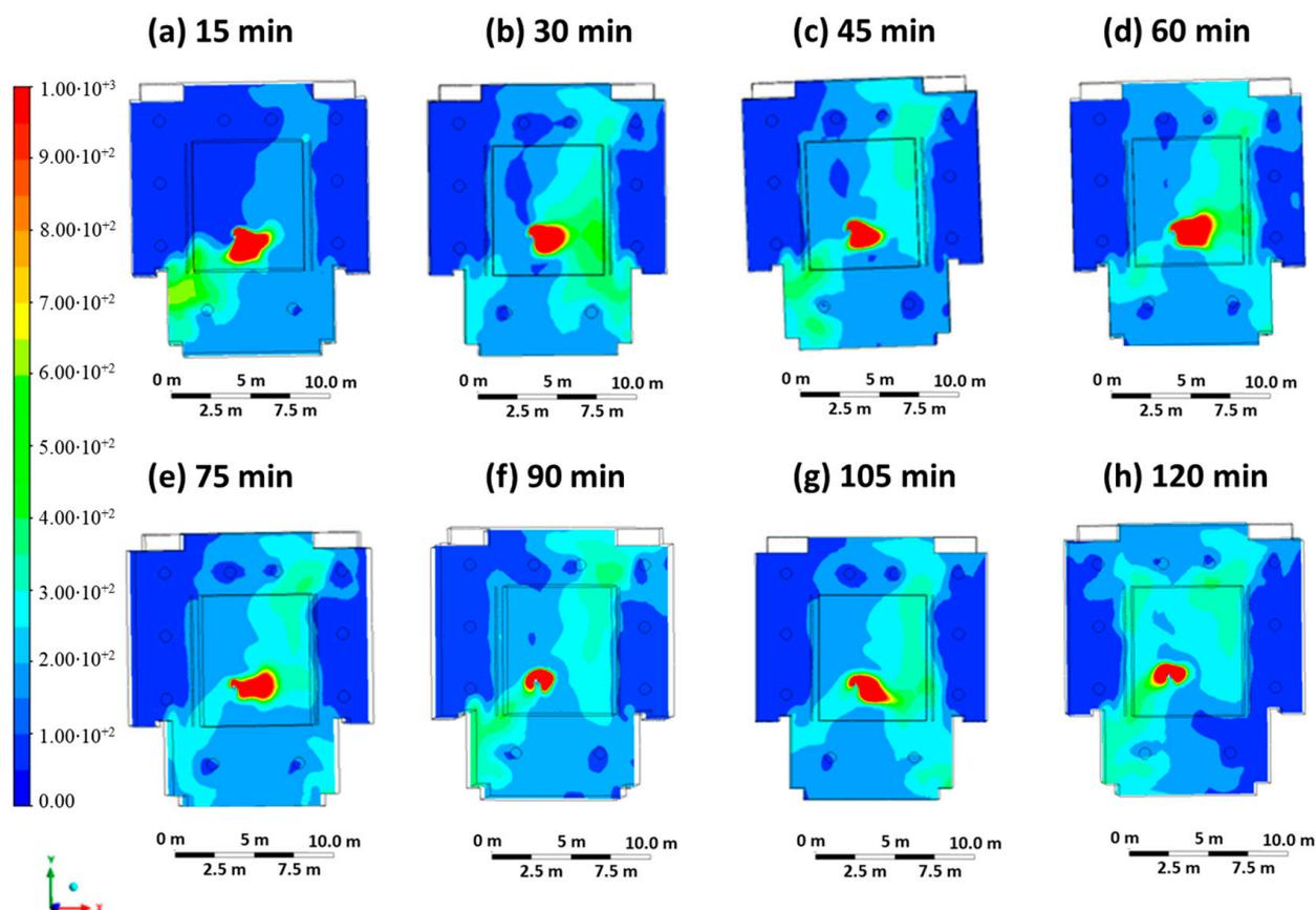
**Figure 7.** Contour maps in terms of carbon dioxide concentration obtained every 15 min in Case 4.
