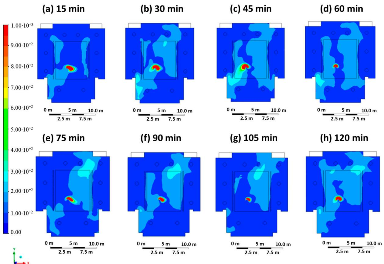
**Figure 8.** Contour maps in terms of carbon dioxide concentration obtained every 15 min in Case 5.
