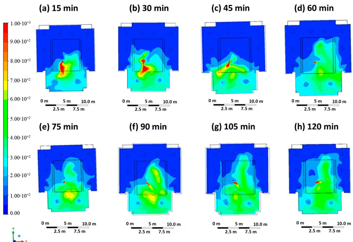
**Figure 6.** Contour maps in terms of carbon dioxide concentration obtained every 15 min in Case 3.
