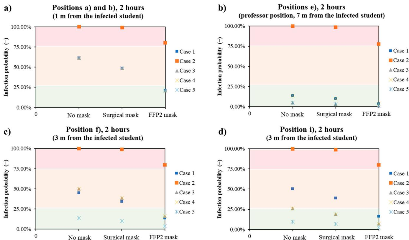
**Figure 9.** Trends of the infection probability in the classroom as a function of the presence of DPI and kind in all the five analyzed cases for different positions: 1 m away from the infected student (a), typical professor position (7 m, (b)), and 3 m away from the infected student (c,d).
