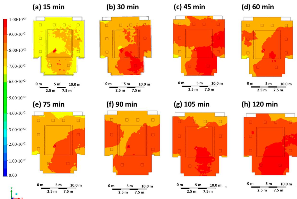
**Figure 5.** Contour maps in terms of carbon dioxide concentration obtained every 15 min in Case 2.
