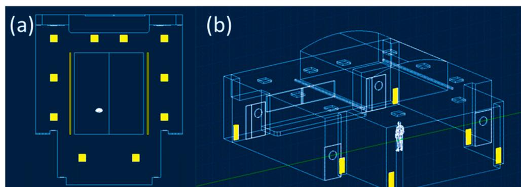
**Figure 2.** The twelve characteristic elements of the supply (a) and return elements of the ventilation system (b) were drawn with Autodesk Autocad 2021 software.
