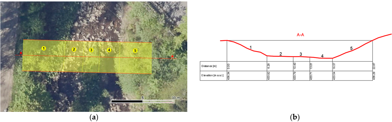
Figure 5. Sample cross-section for roughness coefficient estimation: (a) division into sections of the wetted perimeter with different roughness coefficients, (b) cross-section based on DEM (source: DEM and orthophotomap from maps.geoportal.gov.pl ; accessed on 20 January 2024).
