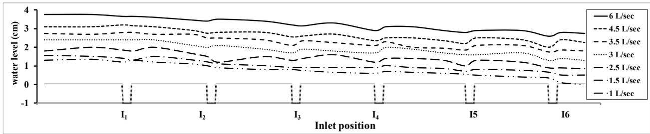
Figure 8. Water surface profile at different inlet discharge rates with six inlets.
