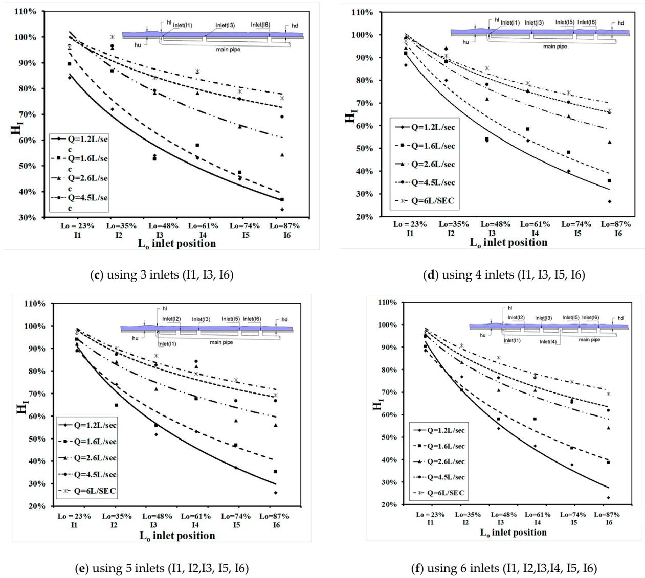
**Figure 9.** Relationship between  $H_I$  and  $L_O$  for different inlet discharge rates.
