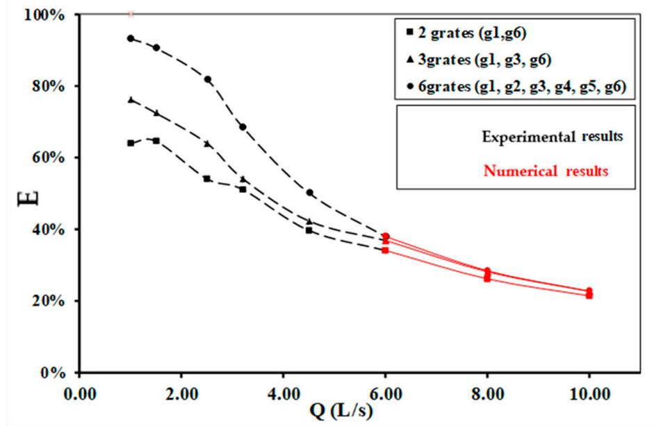
Figure 15. Relationship between total discharge and efficiency when using two, three, and six inlets with different discharges.
