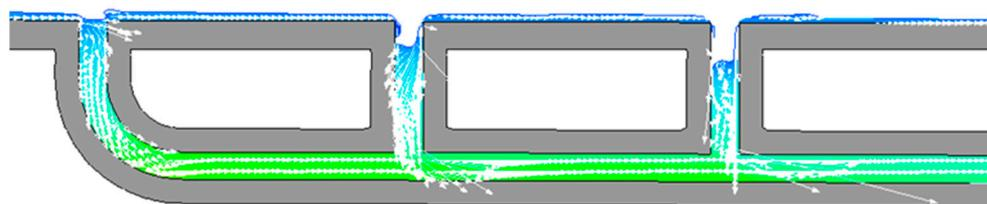
**Figure 13.** Water surface and velocity vector for three grates at  $Q = 2.5\text{L/S}$ .
