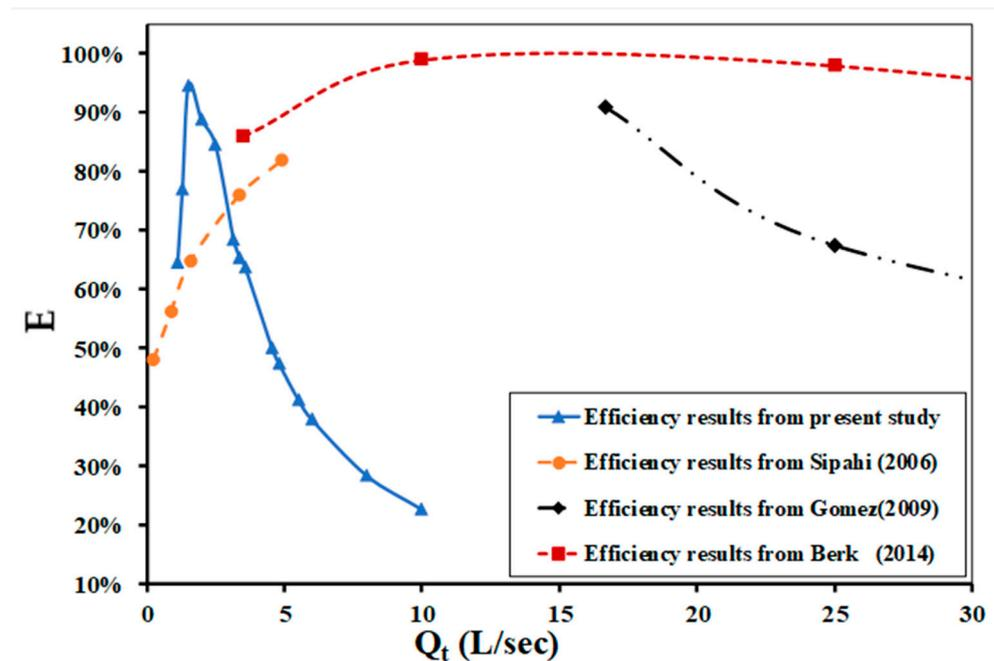
Figure 16. Relationship between total discharge and efficiency for different studies [21–23].
