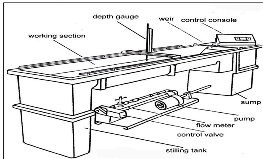
**Figure 2.** Definition sketch of the flume used in the current study.
