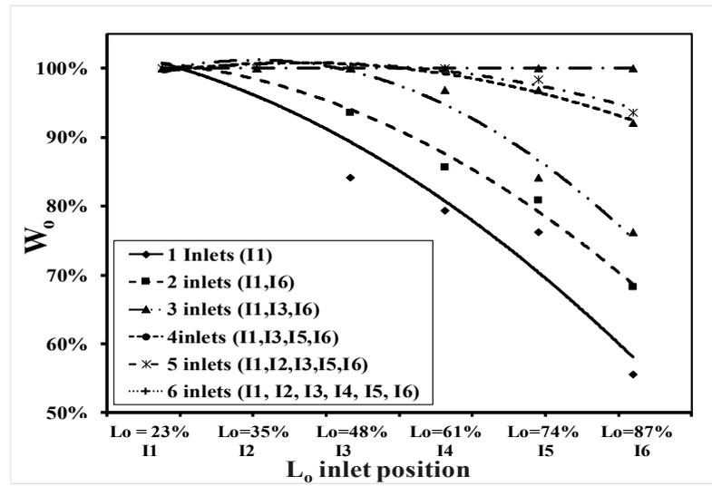
Figure 10. Relationship between relative water spread width and discharge for different numbers of inlets at Q = 1.20 L/S.
