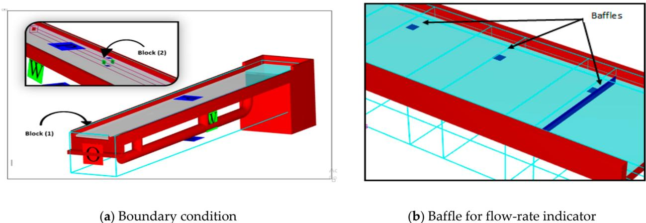
Figure 12. Boundary conditions and baffle for flow-rate indicator.
