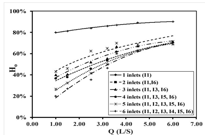
**Figure 7.** Relationship between passing discharge and relative water height with different numbers of inlets.
