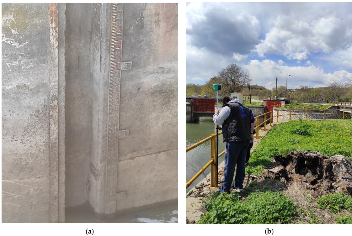
**Figure 7.** (a) an installed water level meter at the gates of the dam that recorded a water depth 0.7 m; (b) the GPS-GNSS antenna RTK "RUIDE NOVA R6" used to obtain the coordinates of the area.
