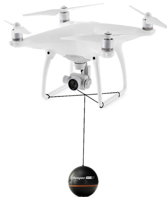
**Figure 4.** The DJI Phantom 4 Pro Unmanned Aerial Vehicle (UAV) coupled with the tethered sonar (Deeper Smart Sonar PRO) for the bathymetric measurements.
