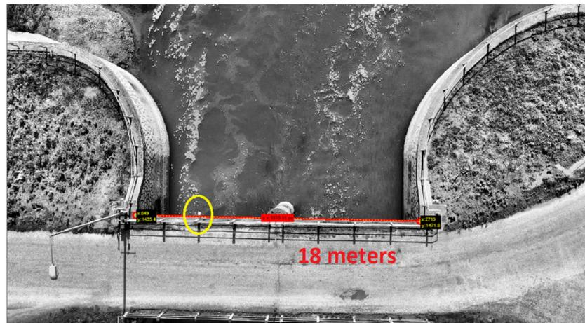
**Figure 9.** The study area of Aggitis section near the Simvoli Dam captured by the UAV parallel to the XY plane. There is a bridge (the main road network) and a telemetric hydrologic station (in the yellow circle) to monitor the streamflow for flood events. The red line (cross-section) is 18 m.
