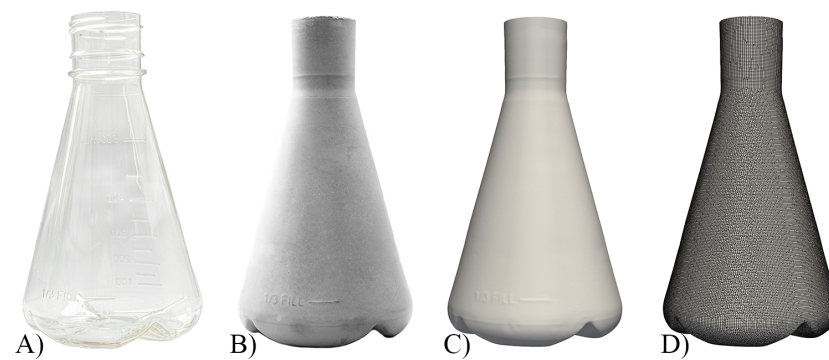
Figure 2. Process steps from the single-use shake flasks to computational mesh. (A) The 500 mL baffled shake flask. (B) Model cast with levelling compound. (C) Scanned and smoothed computer model. (D) Computational mesh used for the CFD simulations.
