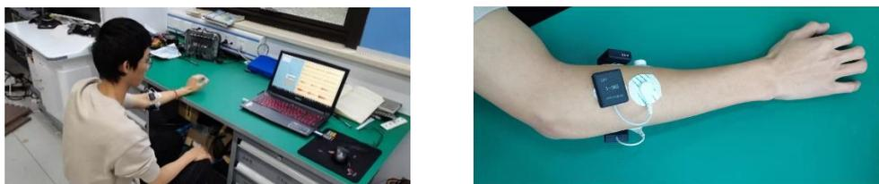
Figure 11. EMG-electrodes placement on the forearm muscles.
