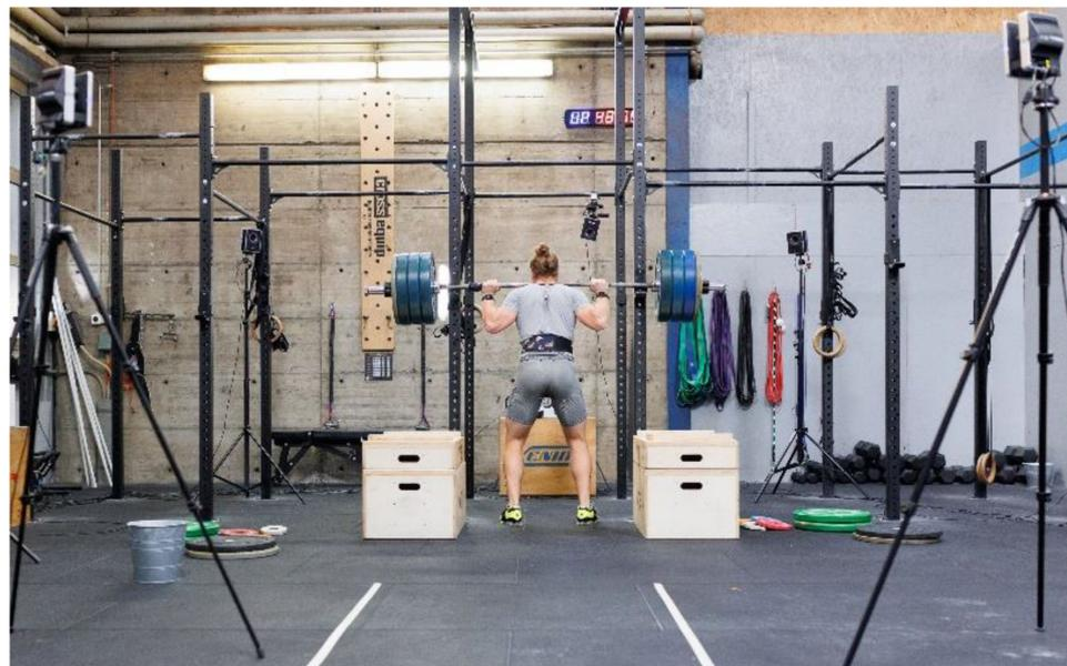
**Figure 2.** A standard rig with a barbell, weight plates, and safety boxes was used for squat performance testing. Kinematic data of squat performance were acquired using a Vicon Motion System (Vantage 5; Vicon Motion Systems Ltd., Oxford, UK) with ten infrared cameras and two markers on each side of the barbell.
