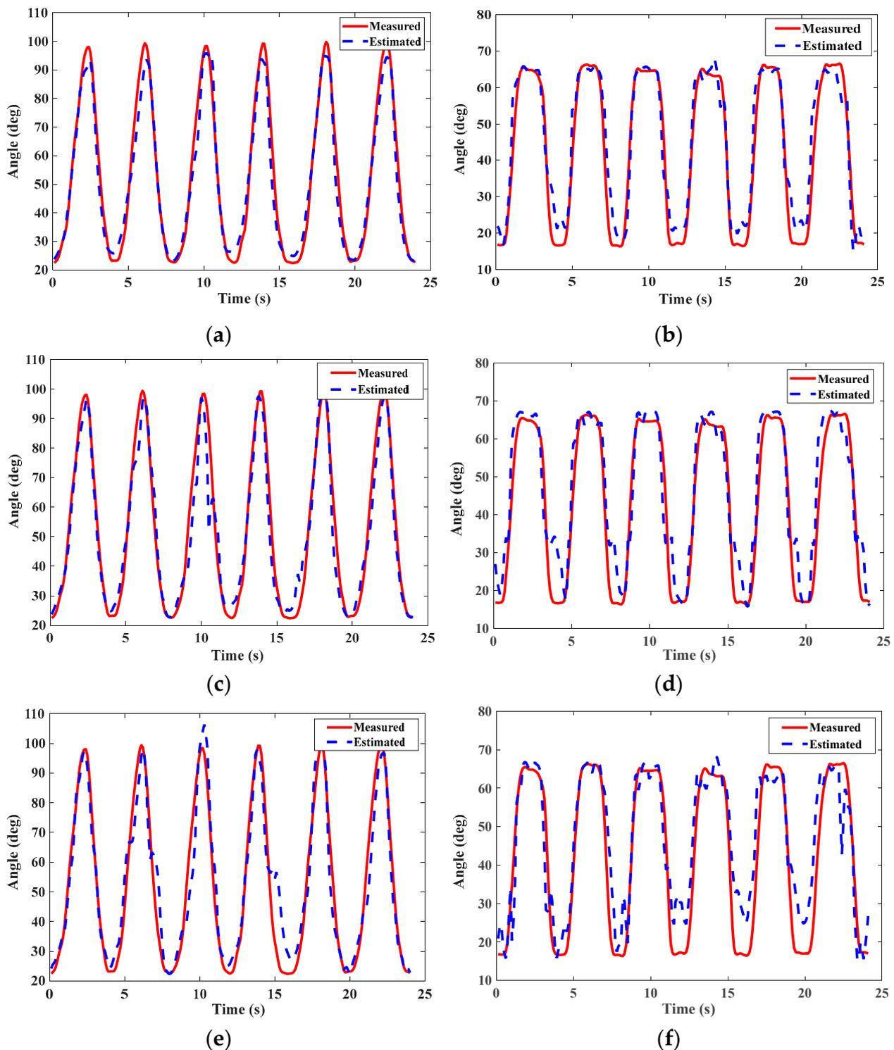
**Figure 11.** (a,c,e) Estimated results of the squat based on PSO-DBN-BP, DBN-BP, and BPNN. (b,d,f) Estimated results of the knee flex/ext based on PSO-DBN-BP, DBN-BP, and BPNN.
