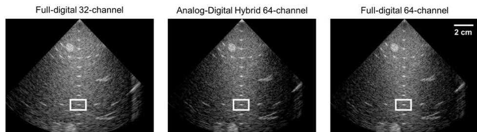
**Figure 10.** Reconstructed B-mode images with three different approaches—32-channel full digital beamforming, 64-channel virtual analog-digital hybrid beamforming, 64-channel full digital beamforming. White rectangles in the images indicate the region-of-interest to measure the lateral resolution.
