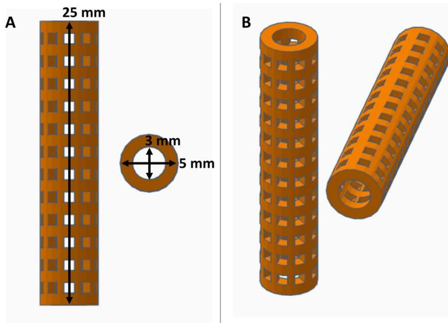
**Figure 1.** Views of computer aided design (CAD) stent with dimensions displayed in orthographic view (A) and in perspective view (B).
