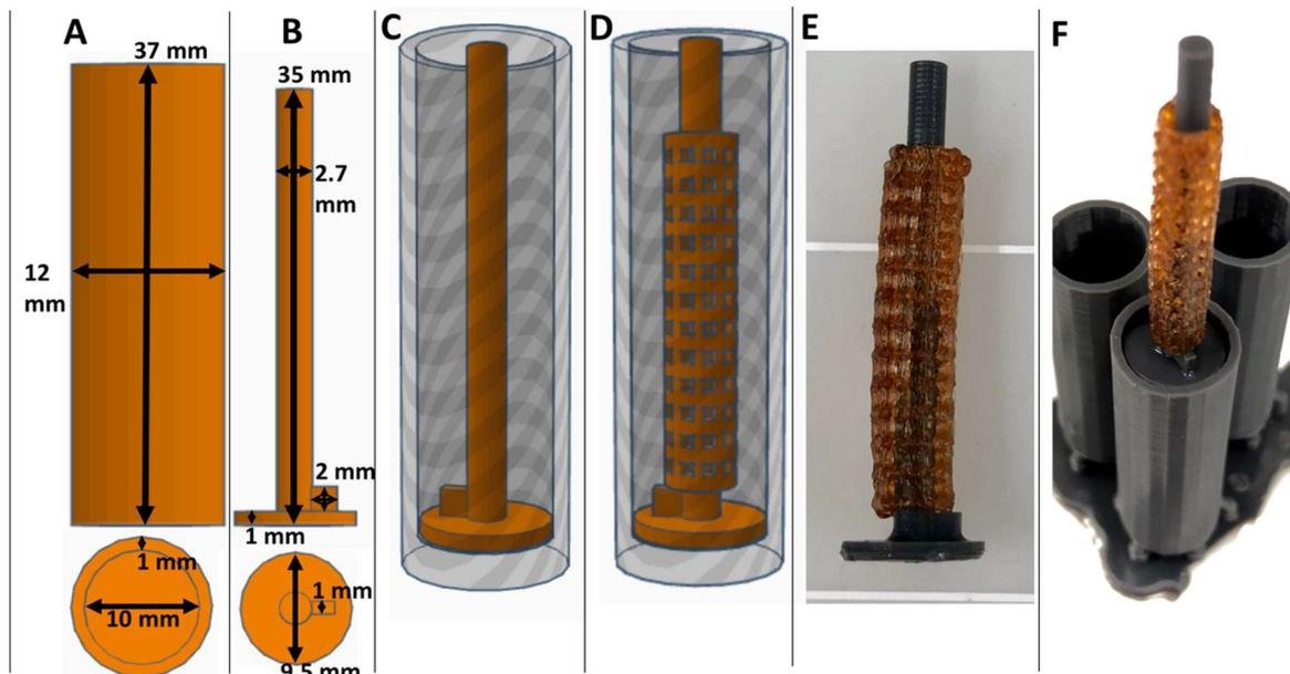
**Figure 2.** Views of CAD collagen injection molding chamber (A) and maturation plug (B) with dimensions displayed. CAD collagen injection molding chamber with maturation plug inserted (C) and with stent placement (D). Images of 3D printed actual crosslinked polyvinyl alcohol (XL-PVA) stents, over a maturation plug (E) and with the injection molding chambers (F).
