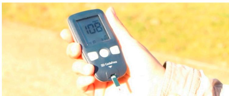
**Figure 4.** A glucose meter is a commercial instrument that uses capillary microfluidics to measure glucose levels in blood droplets. It is operated from a battery and can be used in mobile scenarios.
