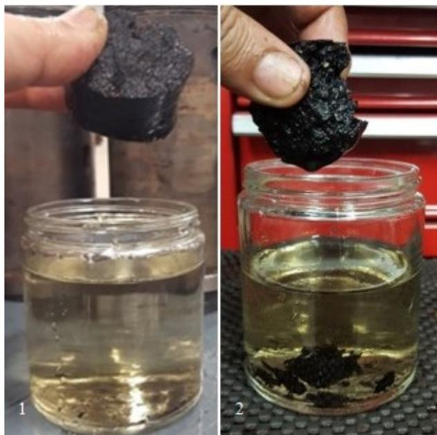
**Figure 13.** After 24 h of water immersion: (1) 10.75% moisture, (2) 16% moisture.
