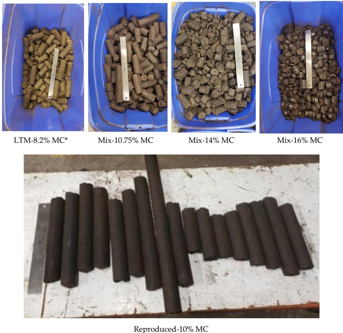
**Figure 5.** Produced briquettes. \* MC: Moisture content (% w.b.).
