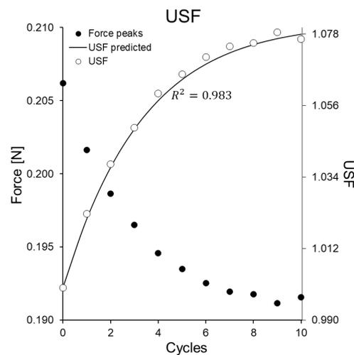
**Figure 6.** Force peaks in stage (2) as a function of the number of cycles performed and USF computed and predicted by Equation (10).
