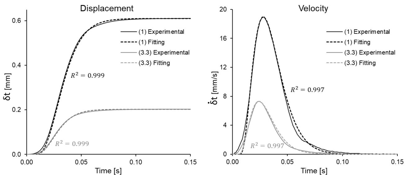
**Figure 3.** Experimental displacement and experimental velocity applied to a specimen, plotted together with the fit by gamma-type function. The plot also shows the derivatives in Sections 1 and 3. It can be seen that the fit is in both cases more extreme than 0.997.
