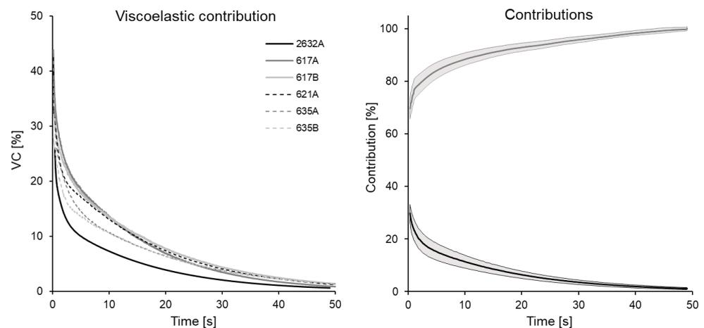
**Figure 5.** Evolution of VC in strength over time for the analyzed specimens: the black lines indicate the average elastic and viscoelastic contributions as a function of time, the shaded area indicates the error interval in the sample.
