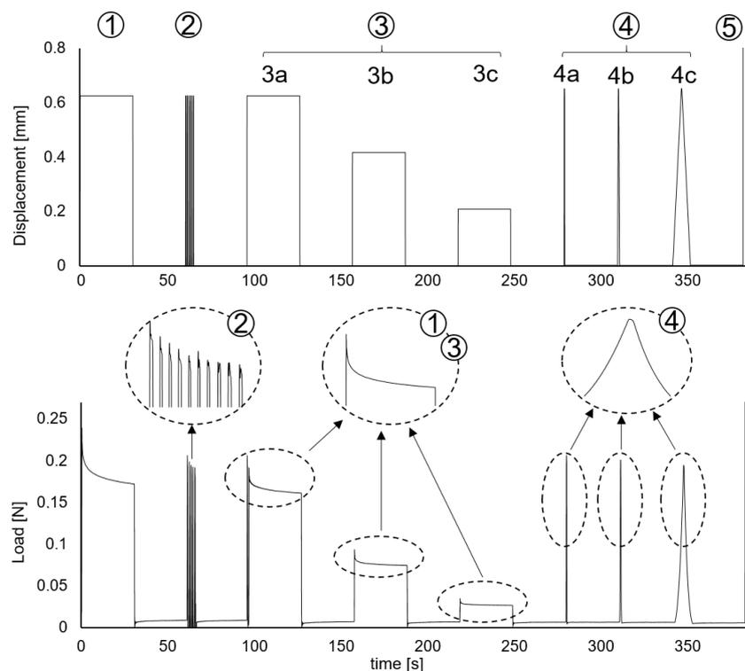
**Figure 2.** Imposed displacements in the different test stages and reaction force of the PSBV for specimen 2632A/20. The stages with constant displacement have been enlarged to show the decrease in force in stages (1) to (3), and the concavity of the load–discharge curve of stage (4).
