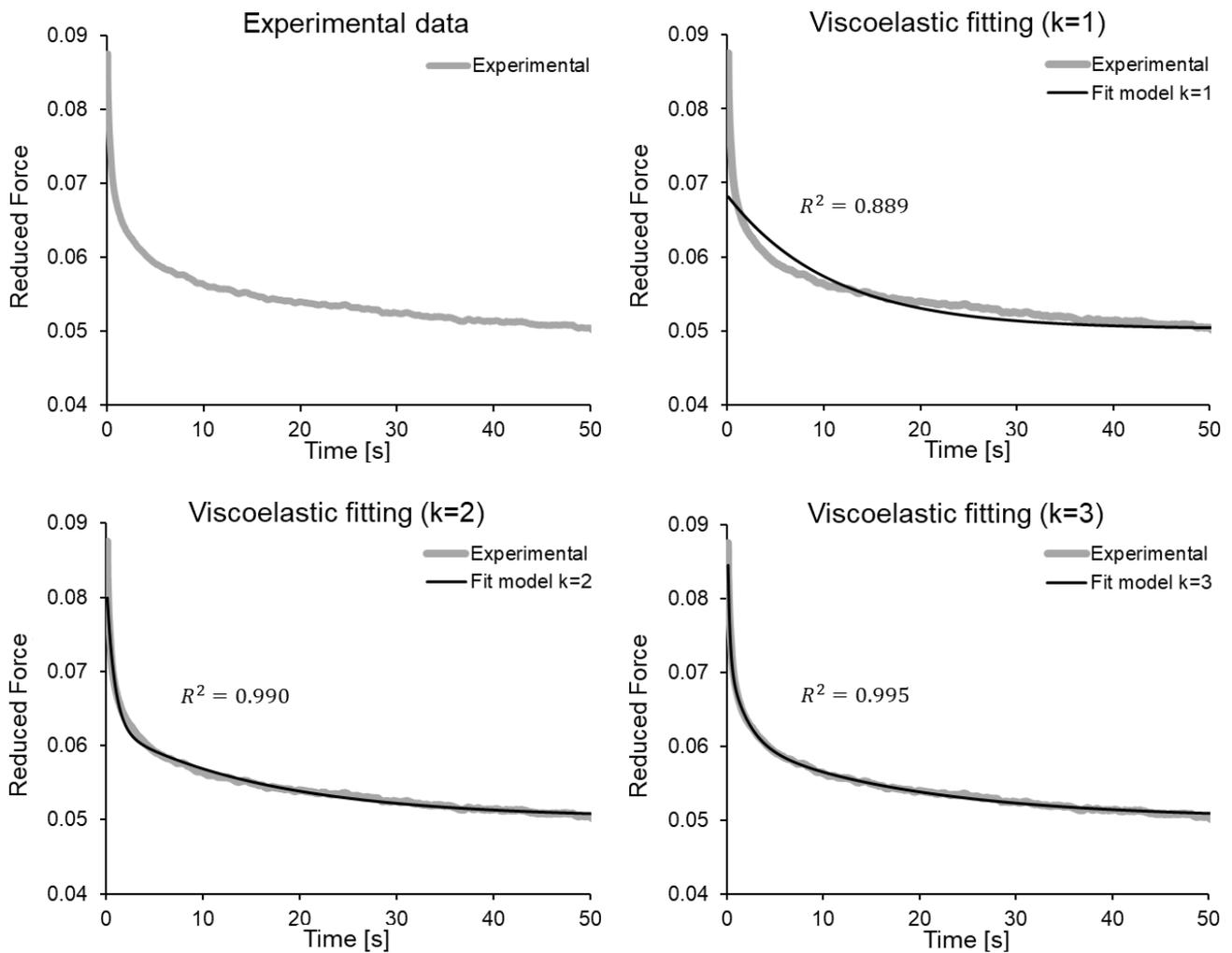
**Figure 4.** Fitting of the proposed viscoelastic model, for stage (1) of one of the specimens. Fits with  $N = 1$ ,  $N = 2$  and  $N = 3$  terms in the Prony series are considered, with the corresponding parameters from Table 1.
