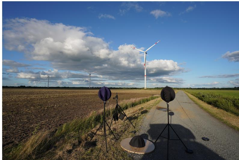
**Figure 6.** The measurement site with the acoustical measurement stations for short-term recordings.
