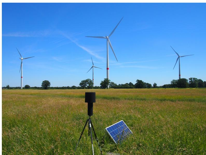
**Figure 5.** The measurement site with one of the acoustical measurement stations and its power supply.
