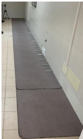
**Figure 2.** GAITFour<sup>®</sup>Dog pressure-sensitive walkway used to perform this study. The PSW is equipped with encapsulated sensor pads available along the entire length of the mat. On each side of the PSW, cameras are positioned at a height of 50 cm. To identify the start and end points of the walk, an inactive mat was placed at each end of the walkway system.
