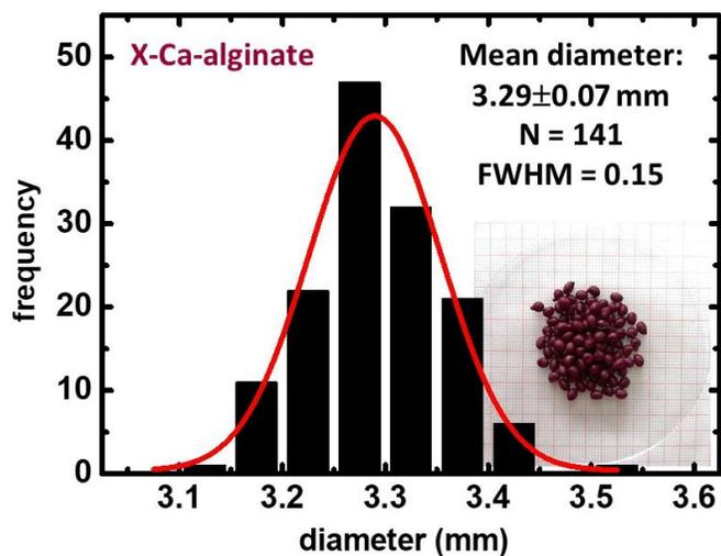
**Figure S1.** Optical photograph and size distribution of X-Ca-alginate aerogel beads (diameters measured with ImageJ); histogram calculated using OriginPro 9.0). Mean diameter and sample size (N) are shown on the Figure.
