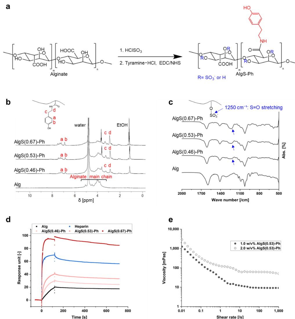
**Figure 2.** Characterization of AlgS-Ph. (a) Reaction scheme for preparing AlgS-Ph. (b)  $^1\text{H}$  NMR spectra of AlgS-Ph ( $\text{D}_2\text{O}$ , 400 MHz). (c) FTIR spectra of AlgS-Ph. (d) SPR analysis of alginate (Alg), AlgS-Ph at various degrees of sulfation and heparin. FGF-2 is immobilized on the sensor surface. (e) Shear-rate–viscosity profiles of solutions containing different concentrations of AlgS(0.53)-Ph (1.0 w/v% and 2.0 w/v%) at 25 °C.
