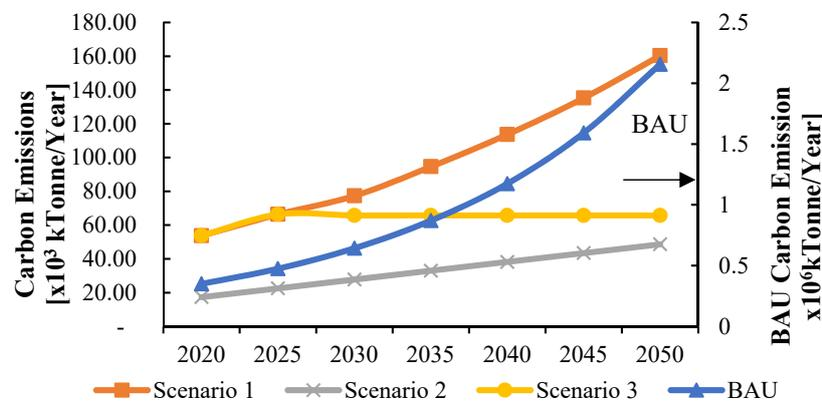
**Figure 7.** Profiles of carbon emissions under BAU and carbon mitigation scenarios. (Scenario 1: Ban on oil use in power generation, Scenario 2: CO<sub>2</sub> price \$7.3/tonne that rises 5% annually, Scenario 3: CO<sub>2</sub> cap by 15% of Scenario 1 by 2030 combined with a ban on oil in power generation).
