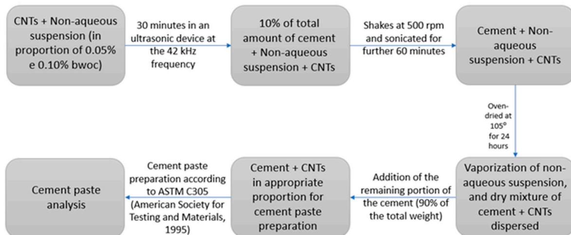
**Figure 3.** Flowchart of the dispersion process of the CNTs in the anhydrous cement particles in a non-aqueous suspension [25].
