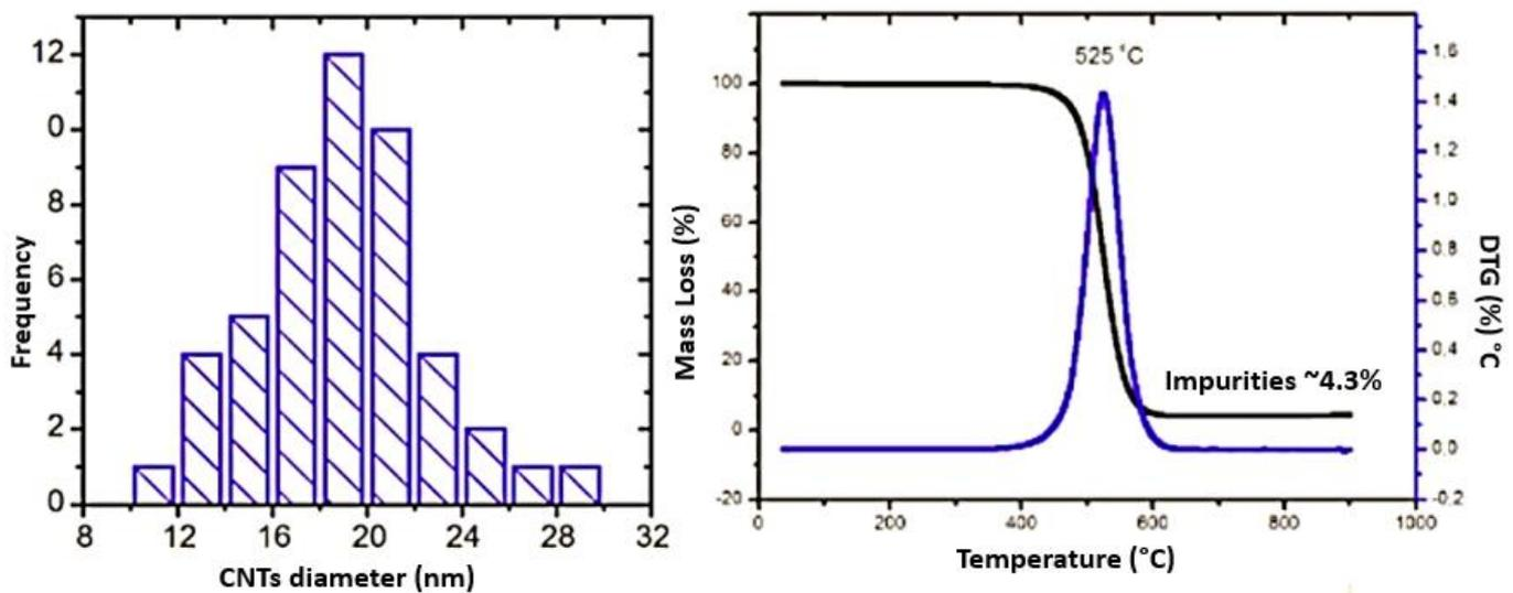
**Figure 2.** Characterization of dimensions and purity information of the CNTs, provided by the supplier.
