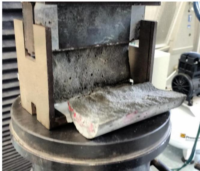
**Figure 5.** Splitting tensile strength test setup.
