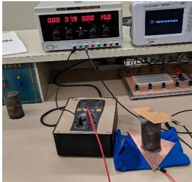
**Figure 4.** Experimental setup of the electric-volumetric resistivity test.
