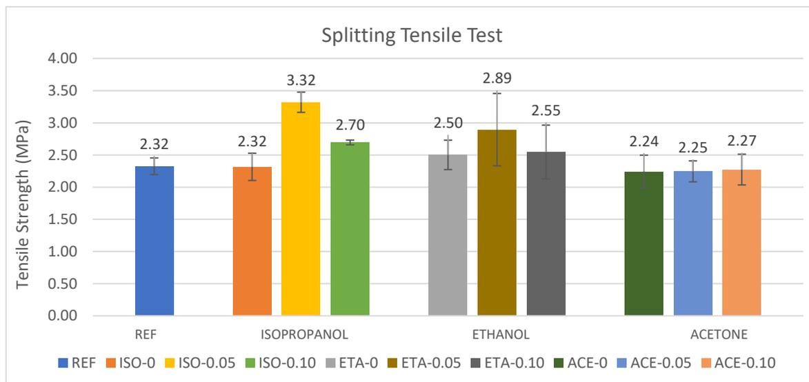
Figure 8. Results of splitting tensile strength tests.
