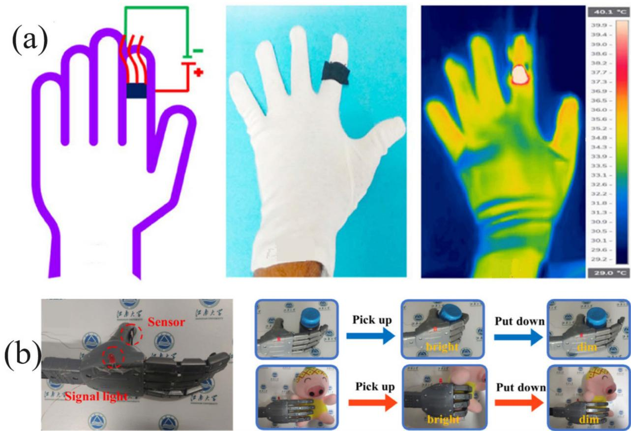
**Figure 14.** (a) Demonstration of the wearable heating system, attachment of the composite with a hand glove as a wearable heater; temperature response of the heater on the index finger under 2 V [121]. (b) PSKF@rGO/SiO<sub>2</sub>-PDMS sensor mounted on a robot hand for executing dangerous tasks and intelligent logistics [102]. The background of Figure 14b is the university name for the author in reference [111].
