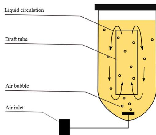
**Figure 4.** Airlift bioreactor design.
