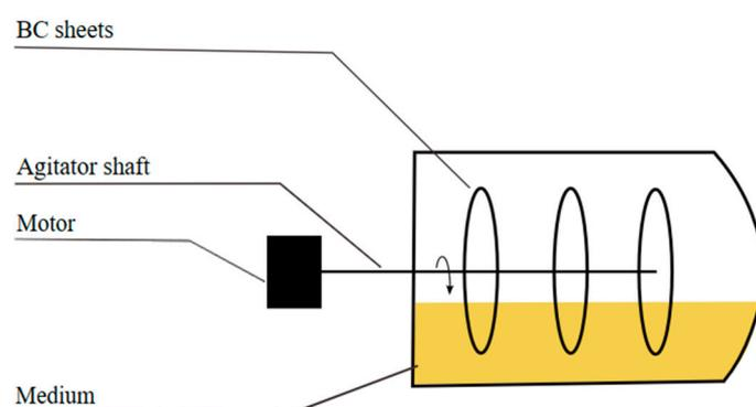
**Figure 5.** Rotating disk bioreactor design.
