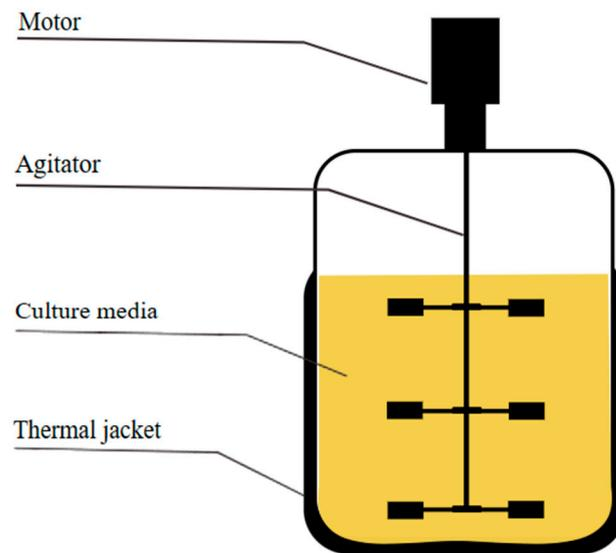
**Figure 3.** Stirred tank bioreactor design.
