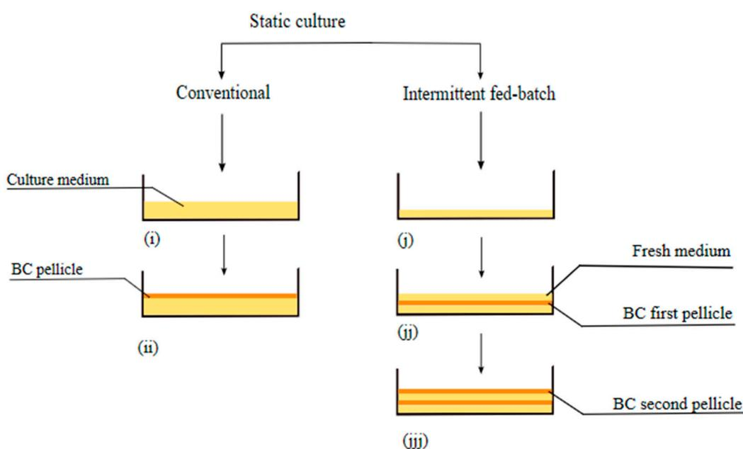
**Figure 2.** Schematic diagram of BC culture. Conventional static culture: (i) substantial amounts of medium are being fed all at once, (ii) only one layer of a BC sheet can be obtained. Intermittent fed-batch culture: (i) a certain amount of medium being fed gradually, (ii) fresh batch of the medium being fed after first BC layer is formed, (iii) another layer of BC is formed, and another fresh medium will, subsequently, be fed.
