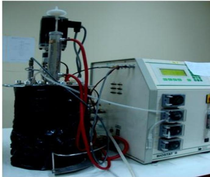
**Figure 6.** Cultivation of *S. limacinum* ATCC MYA-1381 in a 5 L fermenter under the dark condition.
