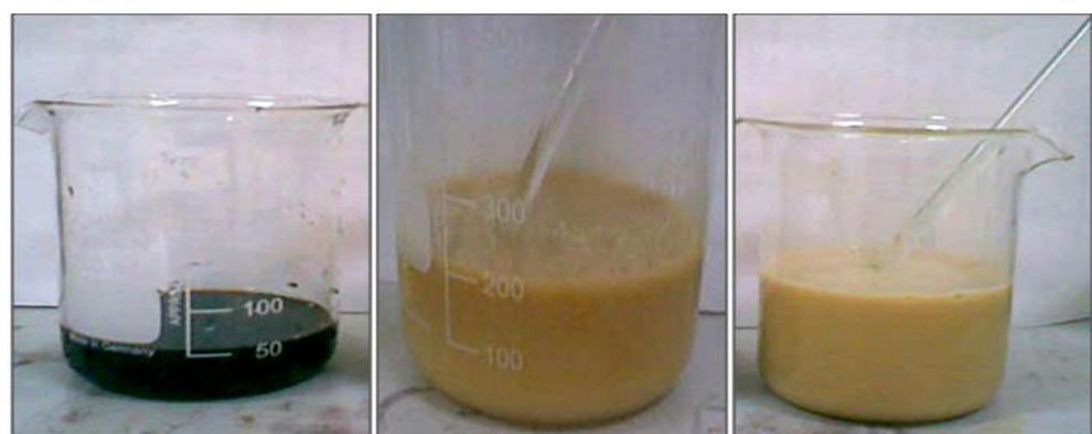
**Figure 3.** (Left) the BDWG before treatment (middle) the BDWG separated from the soap layer when it was mixed in culture medium and (right) the BDWG after treatment.
