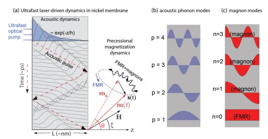
**Figure 1.** (a) Femtosecond laser excitation of a freestanding nickel membrane generates the thermal strain  $\propto \exp{-z/h}$  launching acoustic pulses and precessional magnetization dynamics. Both dynamics can be decomposed in (b) acoustic phonon modes and (c) magnon modes.
