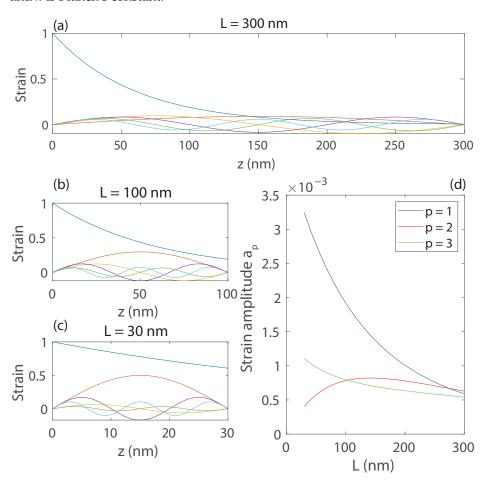
**Figure 2.** Illustration of the first few acoustic eigenmode profiles (normalized) for (a) L = 300 nm, (b) L = 100 nm and (c) L = 30 nm. In each graph, the blue line indicates the overall strain profile, while the other lines indicate the eigenmode components with their respective amplitudes. (d) Strain amplitudes  $a_v(L)$ , for the first three modes p = 1, 2, 3.
