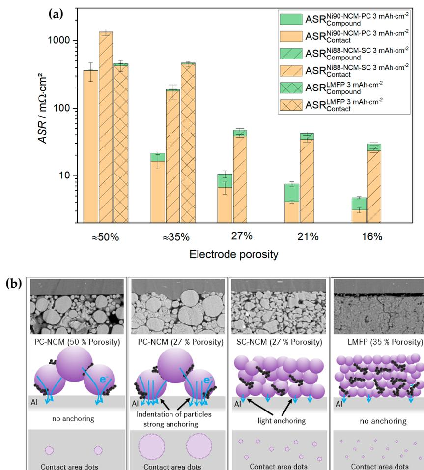
**Figure 8.** (a) Impacts of different electrode porosities from results obtained from 46-point probe electronic resistance measurements. (b) SEM pictures and schematic representations of differences in particle-current collector contact, including the indication of the anchoring of NCM particles into the Al-CC. Please note that the gap between the Al-CC and LMFP coating is an artefact of sample preparation for the cross-section SEM.
