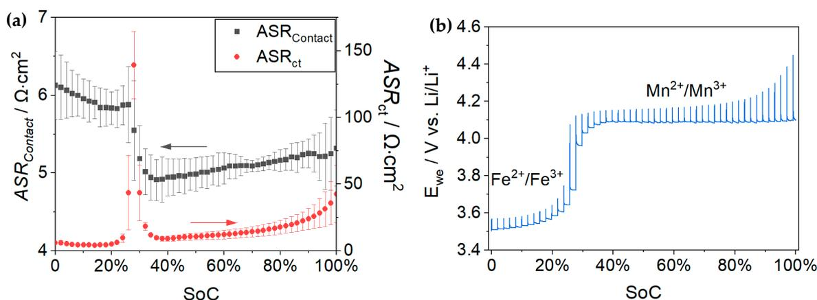
**Figure 2.** (a) Changes in  $R_{\text{Contact}}$  and  $R_{\text{ct}}$  over SoC steps of 2% for a calendered LMFP cathode (porosity: 50%) on the Al-CC, calculated from fitting of EIS data. The error bars indicate the standard deviation of three cells. (b) Characteristic cathode voltage for a measurement in the charge direction, showing the  $\text{Fe}^{2+}/\text{Fe}^{3+}$  and  $\text{Mn}^{2+}/\text{Mn}^{3+}$  redox plateaus of LMFP cathode.
