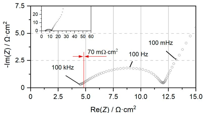
**Figure 7.** EIS plot of Ni90-NCM-PC (porosity: 27%) coated on an Al-CC measured at a 25 °C and 50% SoC. The contribution of  $R_{\text{Contact}}$  is negligible. The thickness of the red line indicates the possible magnitude of  $R_{\text{Contact}}$ , assuming it would be 10 times the value measured using the 46-point probe method. The inset shows a zoom out of the same Nyquist plot; a continuation of the capacitive tail can be observed.
