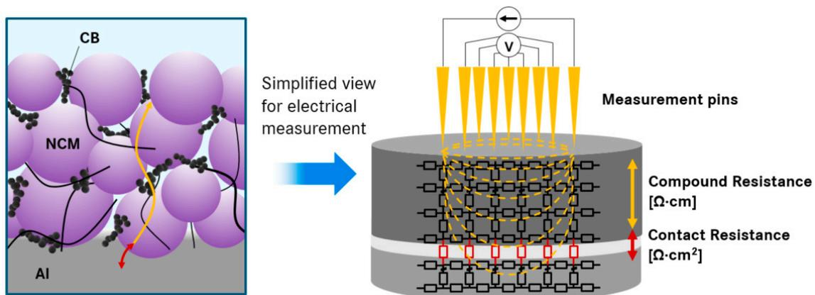
**Figure 5.** Schematic representation of the resistance types received from the 46-point probe measurement.
