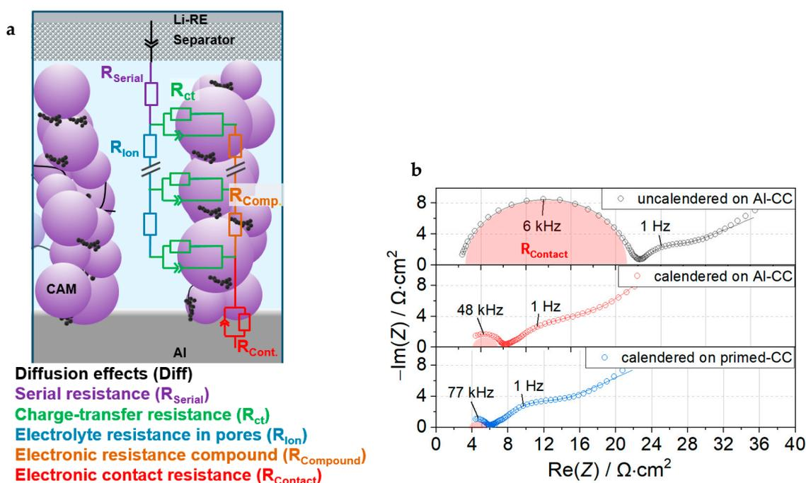
**Figure 1.** (a) Scheme of transmission line model-based equivalent circuit used for impedance measurement fittings in this work (b) EIS spectra of LMFP cathodes with varying calendering grades and current collectors at 0% SoC after formation. Presumed  $R_{\text{Contact}}$  contributions are highlighted with red semi-circles. Continuous lines indicate fitting results.
