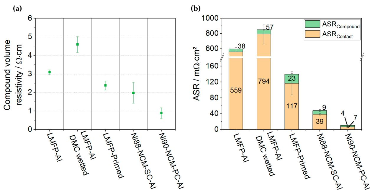
**Figure 6.** (a) The 46-point probe results for compound volume resistivity ( $R_{\text{Compound}}$ ). (b) Comparison of the ASR obtained from 46-point probe measurements for samples with porosities of 50% for LMFP cathodes and 27% for NCM cathodes. The transformation to  $\text{ASR}_{\text{Compound}}$  was performed through normalization to sample thickness.
