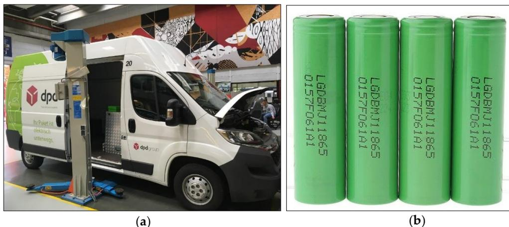
Figure 1. (a) The eVan20, the project demonstrator, and (b) the LG MJ1 cells of the battery pack.
